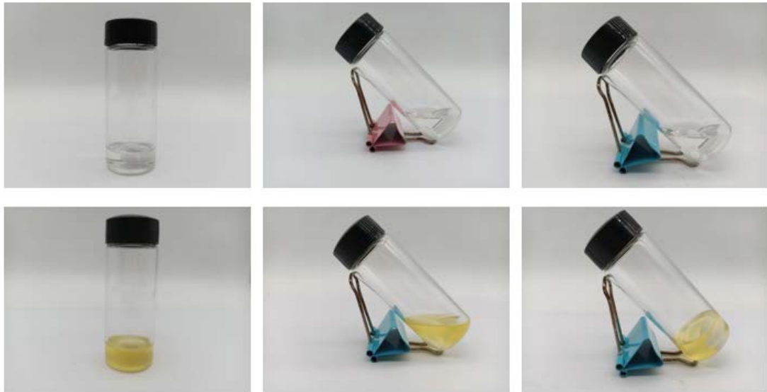
Fig. S1. Optical image of heating crosslinking process of polymer blends (top) and TA-hybrid network (bottom)
