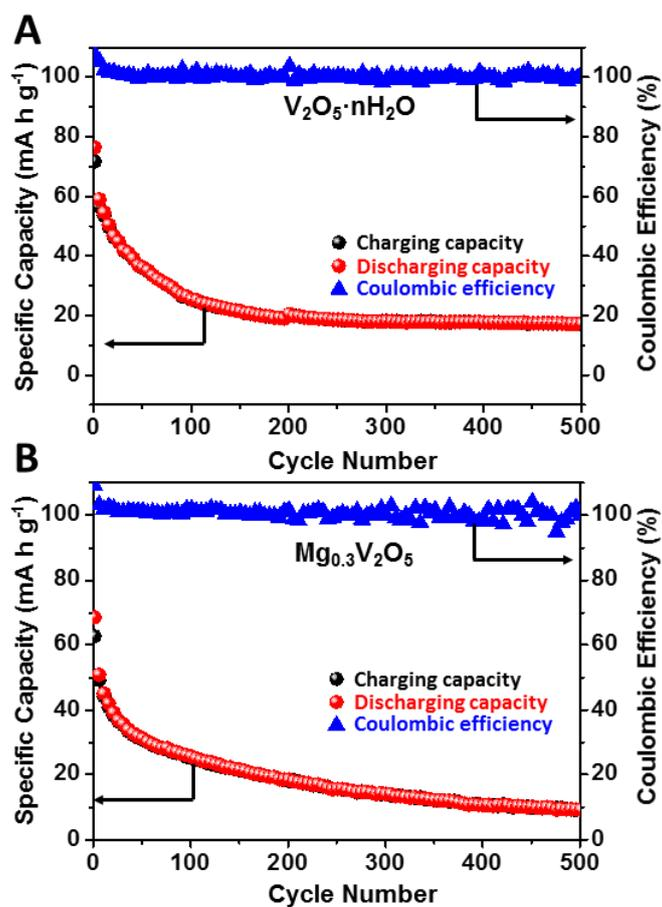
**Figure S10.** Cycling performances of (A)  $\text{V}_2\text{O}_5 \cdot n\text{H}_2\text{O}$  and (B)  $\text{Mg}_{0.3}\text{V}_2\text{O}_5$  at  $0.5 \text{ A g}^{-1}$ , respectively.
