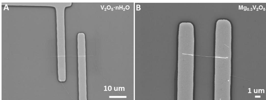
**Figure S11.** SEM images of the (A)  $V_2O_5 \cdot nH_2O$  and (B)  $Mg_{0.3}V_2O_5$  single nanowire devices, respectively.
