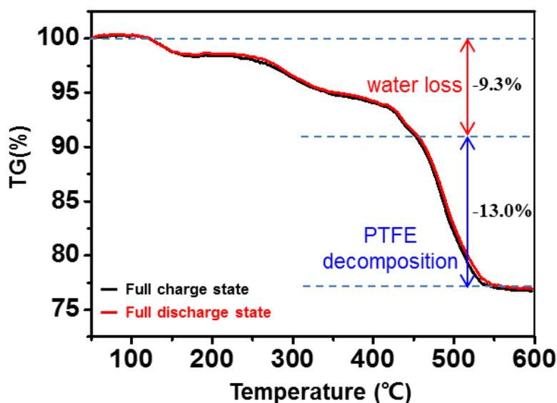
**Figure S14.** Thermogravimetry analysis (TGA) curves of  $\text{Mg}_{0.3}\text{V}_2\text{O}_5 \cdot 1.1\text{H}_2\text{O}$  nanowires after charging and discharging.
