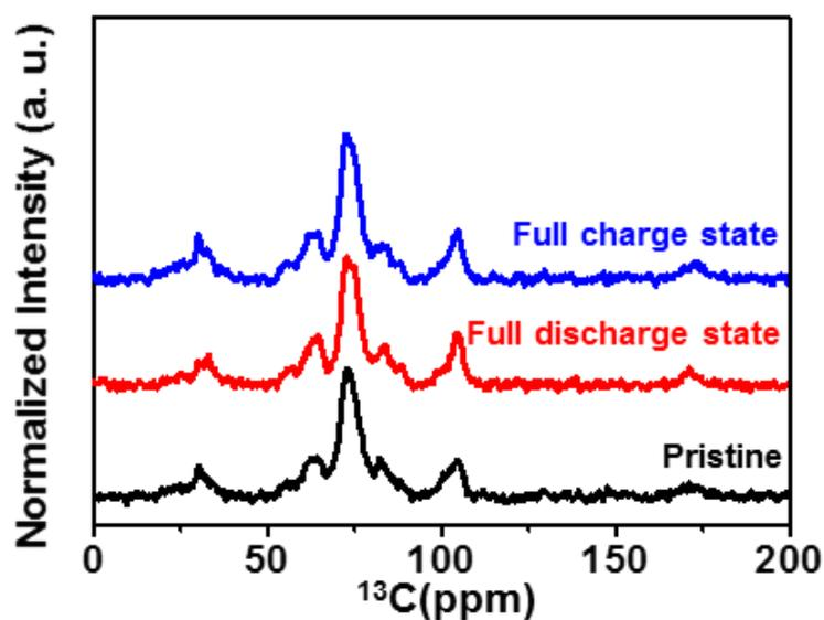
**Figure S15.**  $^{13}\text{C}$  MAS NMR spectra collected for pristine  $\text{Mg}_{0.3}\text{V}_2\text{O}_5 \cdot 1.1\text{H}_2\text{O}$  (black line),  $\text{Mg}_{0.3}\text{V}_2\text{O}_5 \cdot 1.1\text{H}_2\text{O}$  after full discharging (red line) and full charging (blue line).
