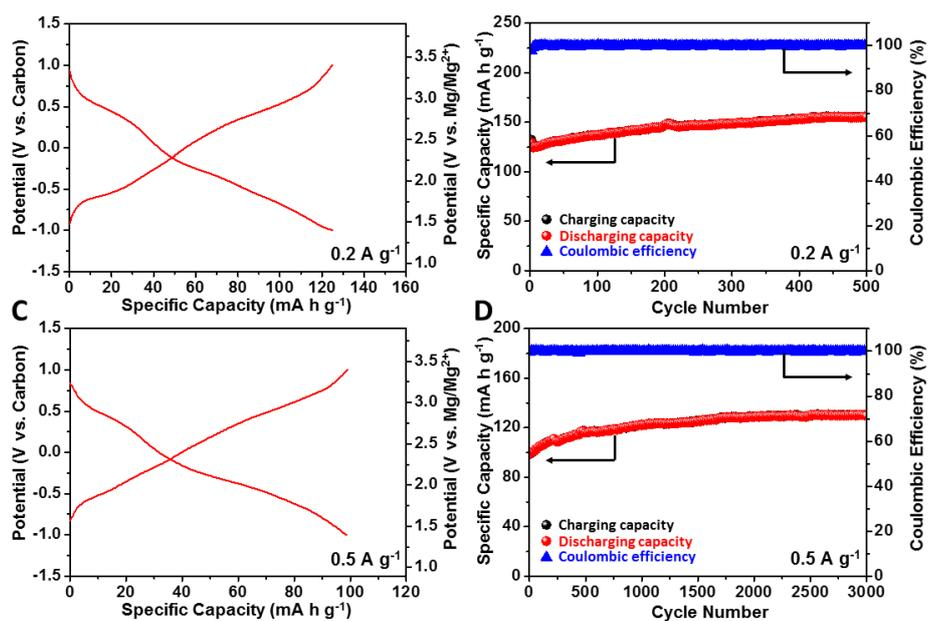
**Figure S9.** Discharge-charge curves (A,C) and cycling performances (B,D) of  $\text{Mg}_{0.3}\text{V}_2\text{O}_5 \cdot 1.1\text{H}_2\text{O}$  at  $0.2$  and  $0.5 \text{ A g}^{-1}$ , respectively.
