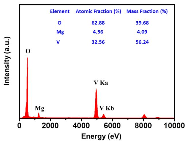
**Figure S4.** Energy dispersive X-ray (EDX) spectrum of the  $\text{Mg}_{0.3}\text{V}_2\text{O}_5 \cdot 1.1\text{H}_2\text{O}$ .
