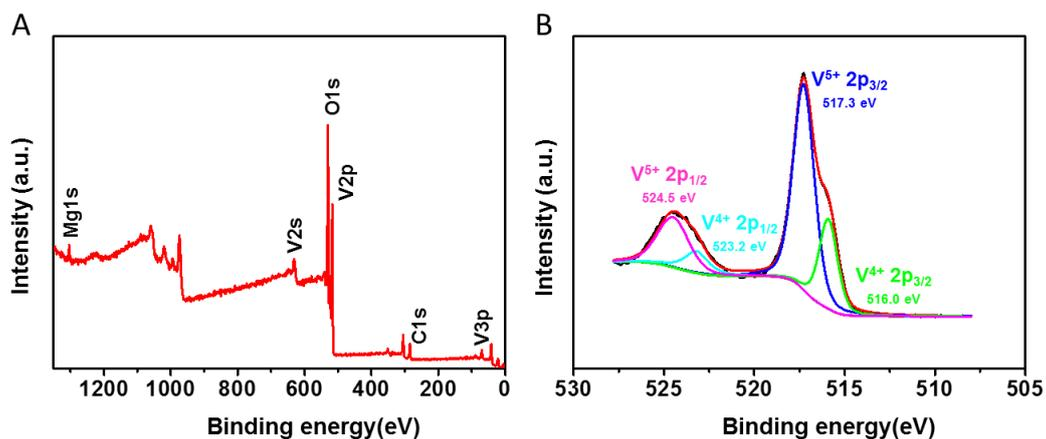
**Figure S3.** (A) Survey XPS spectrum and (B) high-resolution XPS spectrum of V2p peak for the resulting  $\text{Mg}_{0.3}\text{V}_2\text{O}_5 \cdot 1.1\text{H}_2\text{O}$ .
