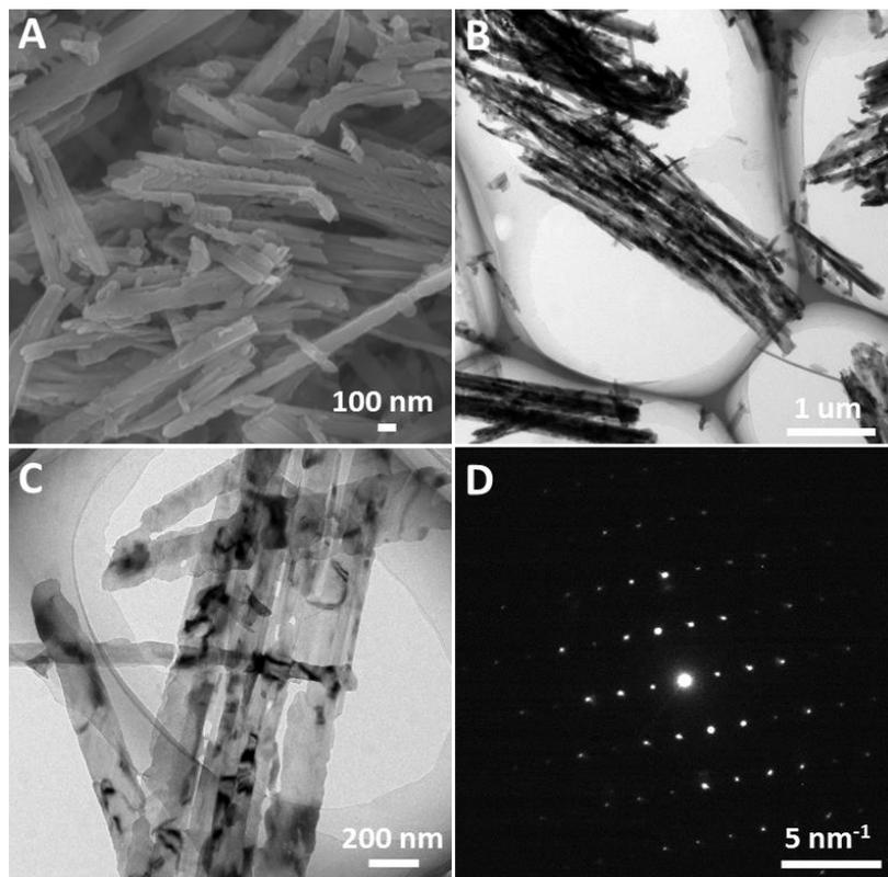
**Figure S6.** (A) FESEM image, (B,C) TEM images, (inset of C) HRTEM image and (D) SAED pattern of  $\text{Mg}_{0.3}\text{V}_2\text{O}_5$ .
