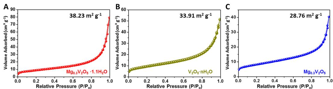
**Figure S7.** Nitrogen adsorption-desorption isotherms of (A)  $\text{Mg}_{0.3}\text{V}_2\text{O}_5 \cdot 1.1\text{H}_2\text{O}$ , (B)  $\text{V}_2\text{O}_5 \cdot n\text{H}_2\text{O}$  and (C)  $\text{Mg}_{0.3}\text{V}_2\text{O}_5$ .
