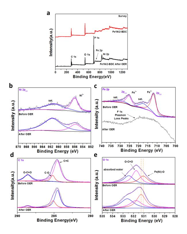
**Figure S11.** XPS characterization of Fe1Ni2-BDC and corresponding catalysts after 2 h durability test in 1 M KOH: (a) survey, (b) Ni 2p, (c) Fe 1s, (d) C 1s and (e) O 1s XPS spectra.
