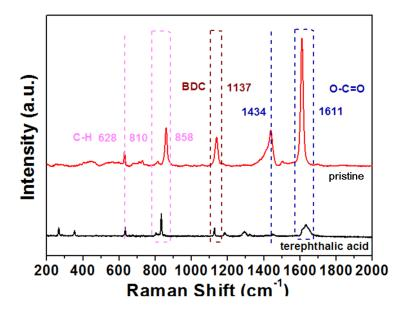
Figure S1. Raman spectra of Fe1Ni2-BDC and terephthalic acid.
