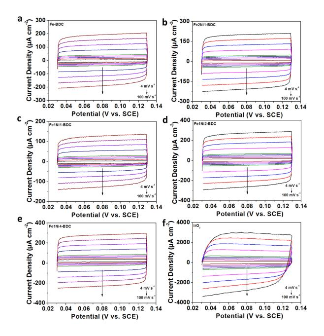
**Figure S7.** CV curves of (a) Fe-BDC, (b) Fe2Ni1-BDC, (c) Fe1Ni1-BDC, (d) Fe1Ni2-BDC, (e) Fe1Ni4-BDC and (f)  $IrO_2$  at different scan rates from 4 to 100 mV s<sup>-1</sup>.
