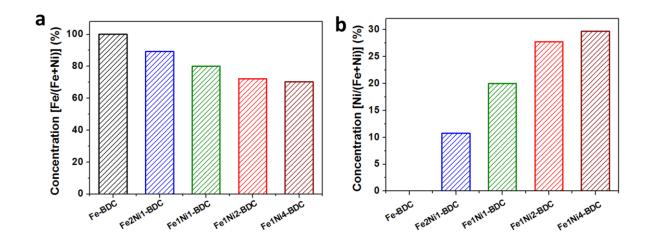
**Figure S2.** ICP analysis of Fe-BDC, Fe2Ni1-BDC, Fe1Ni1-BDC, Fe1Ni2-BDC and Fe1Ni4-BDC: (a) concentration of Fe, calculated by Fe/(Fe+Ni); (b) concentratiosn of Ni, calculated by Ni/(Fe+Ni).
