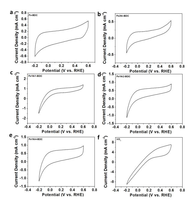
**Figure S6.** CV curves of (a) Fe-BDC, (b) Fe2Ni1-BDC, (c) Fe1Ni1-BDC, (d) Fe1Ni2-BDC, (e) Fe1Ni4-BDC and (f)  $IrO_2$  in PBS solution (pH = 7.0) at a scan rate of 50 mV s<sup>-1</sup>.
