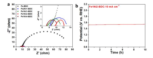
**Figure S9.** (a) The corresponding Nyquist plots of different catalysts, the inset shows enlargement of them. (b) Durability tests of Fe1Ni2-BDC in 1 M KOH at a constant current density of 10 mA cm<sup>-2</sup>.
