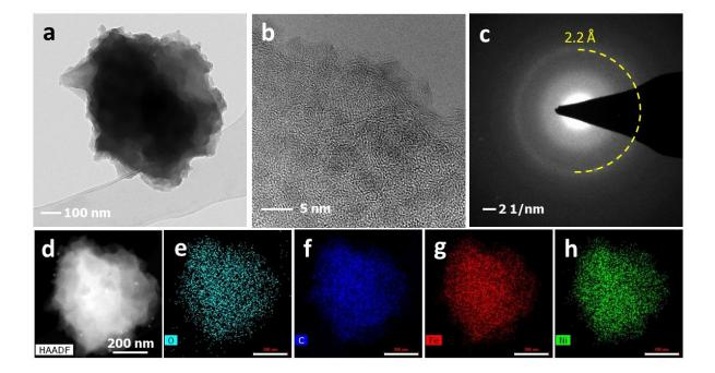
**Figure S10.** (a) TEM image, (b) HRTEM image and (c) SAED pattern, (d) HAADF-STEM image and (e-h) the corresponding EDX elemental maps of the Fe1Ni2-BDC after OER durability test in 1 M KOH for 2 h. Scale bar dimensions in e-h are all 200 nm.
