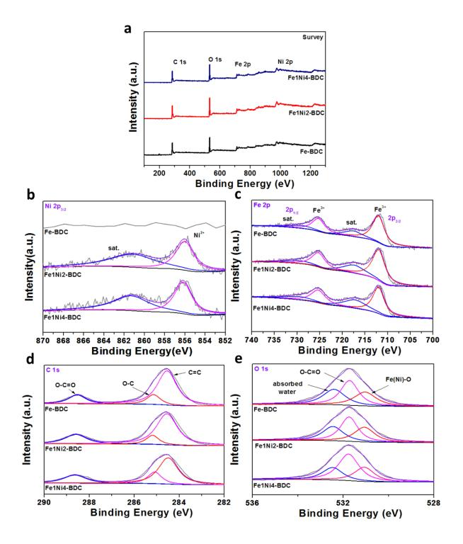
Figure S5. XPS characterization of Fe-BDC, Fe1Ni2-BDC and Fe1Ni4-BDC: (a) survey, (b) Ni 2p, (c) Fe 2p, (d) C 1s and (e) O 1s spectra.
