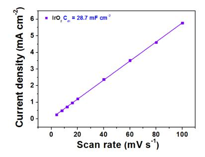
**Figure S8.** CV current density versus scan rate of  $IrO_2$ , the linear slope is equivalent to the double-layer capacitance ( $C_{dl}$ ).
