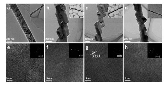
Fig. 3 Morphologies of products synthesized with different amounts of CTAB. TEM images of simple NVO (a), NVO-C1 (b), NVO-C2 (c) and NVO-C3 (d), and the insets in (a-d) show the morphologies in different scales (scale bar for a inset: 200 nm; for b-d insets:  $1 \mu m$ ). HRTEM images of simple NVO (e), NVO-C1 (f), NVO-C2 (g) and NVO-C3 (h), and the corresponding SAED patterns are shown in the insets of (e-h) with zone axis indicated.
