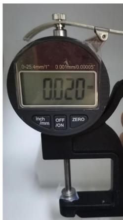
**Figure S1.** Photograph as-prepared flexible GTSSE electrolyte with the thickness of 20  $\mu\text{m}$ .
