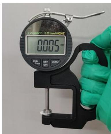
**Figure S3.** Photograph of ultrathin porous membrane with the thickness of 5  $\mu\text{m}$ .
