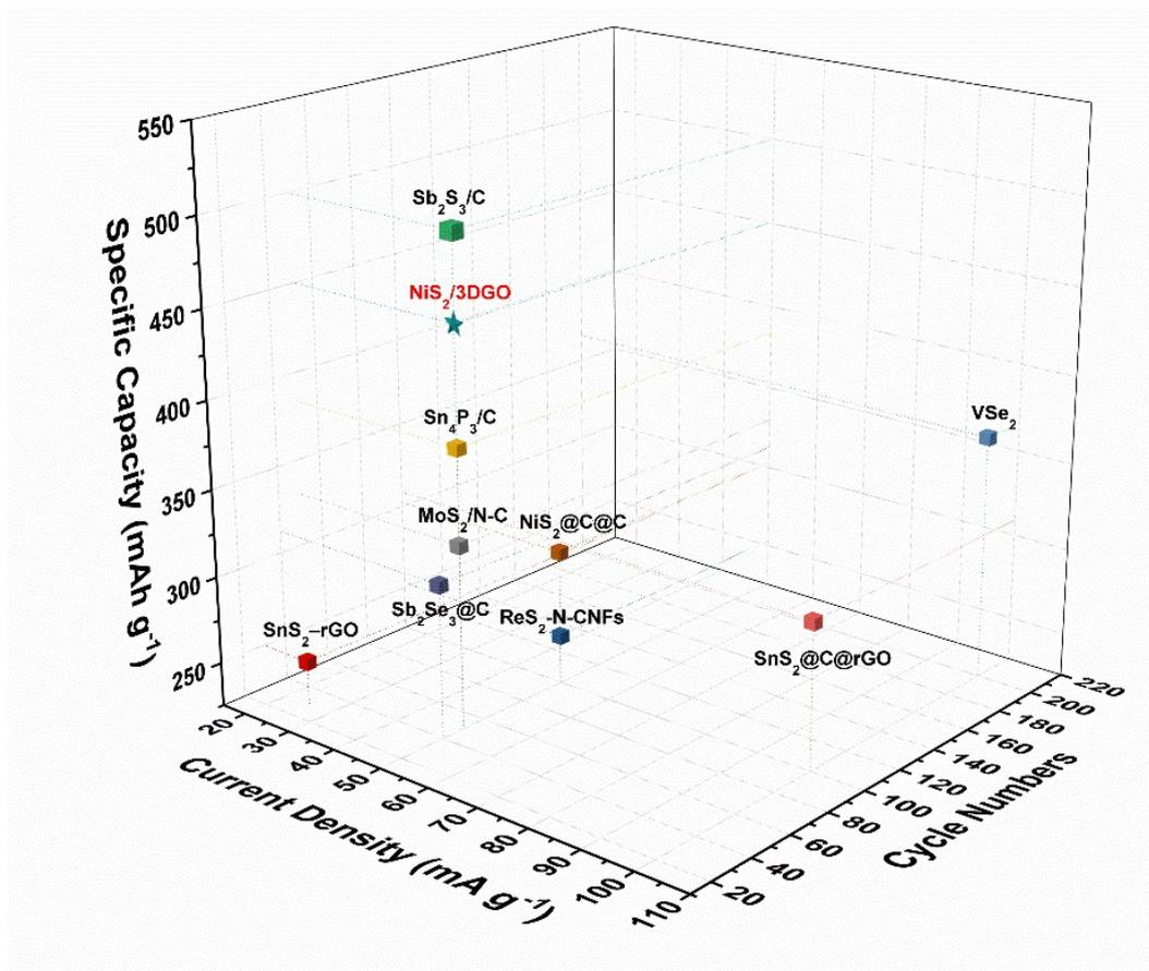
Figure S7. Summary of recent advances on electrode materials and methodologies for PIBs.
