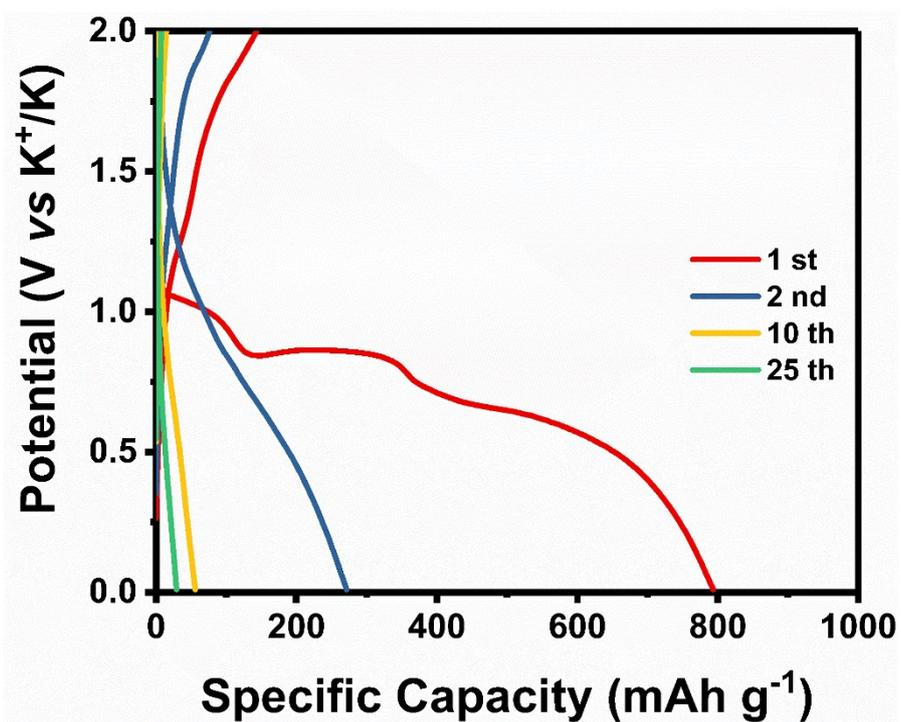
Figure S6. Representative galvanostatic charge–discharge curves of NiS<sub>2</sub> microflowers at 50 mA g<sup>-1</sup>.
