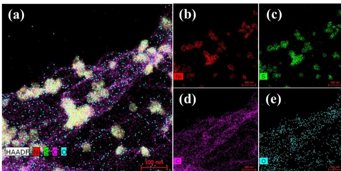
Figure S4. HAADF-STEM image of a) NiS<sub>2</sub>/3DGO with EDS-mapping of b) Ni, c) S, d) C and e) O.
