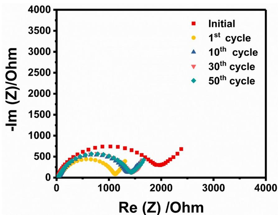
Figure S8. EIS curves after different number of cycles.
