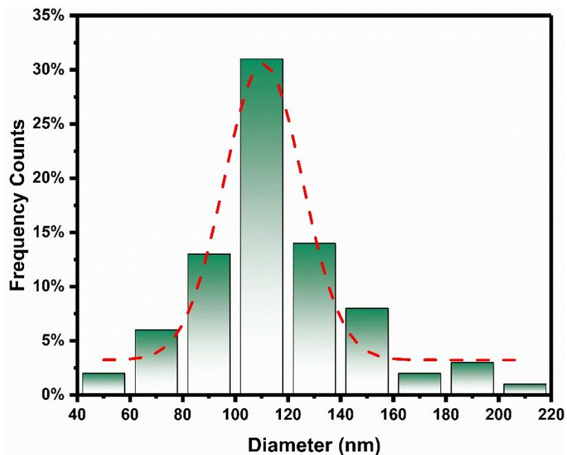
Figure S3. The particle-size distribution (PSD) of the NiS<sub>2</sub>/3DGO
