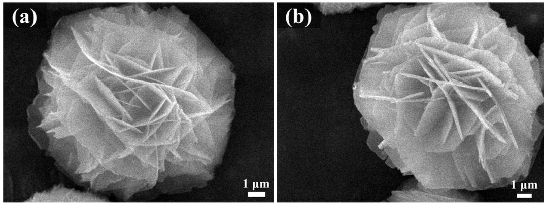
Figure S1. SEM images of nickel-based precursors; a) 6h, b)8h.
