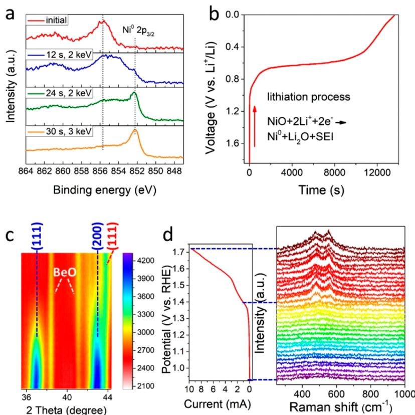
Figure 2. (a) High-resolution depth-sputtering Ni 2p XPS spectra of Ni@NiOOH/NF. (b) First galvanostatic discharging curve of the NiO anode at 300 mA g<sup>-1</sup>. (c) Corresponding in situ XRD patterns showing the conversion reaction of NiO to Ni. (d) Recorded LSV curve and corresponding in situ Raman spectra with a potential interval  $\Delta V$  of 25 mV (0.924–1.724 V<sub>RHE</sub>), revealing the formation of NiOOH after the electro-oxidation process.
