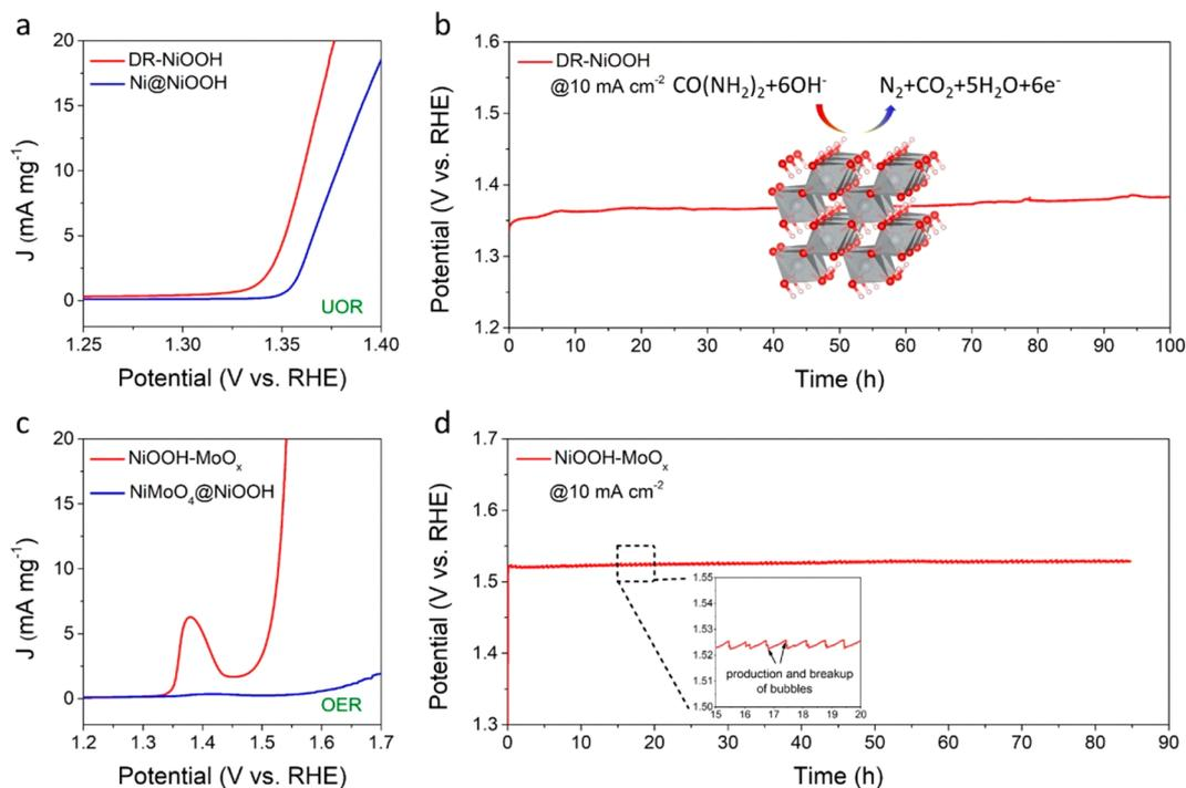
**Figure 5.** (a) UOR polarization curves of DR-NiOOH and Ni@NiOOH normalized by mass. (b) Chronopotentiometry measurement of DR-NiOOH. (c) Mass activity of NiOOH-MoO<sub>x</sub> and NiMoO<sub>4</sub>@NiOOH. (d) Chronopotentiometry measurement of NiOOH-MoO<sub>x</sub>.
