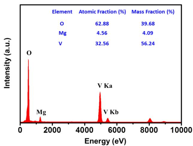
**Figure S4.** Energy dispersive X-ray (EDX) spectrum of the  $\text{Mg}_{0.3}\text{V}_2\text{O}_5 \cdot 1.1\text{H}_2\text{O}$ .
