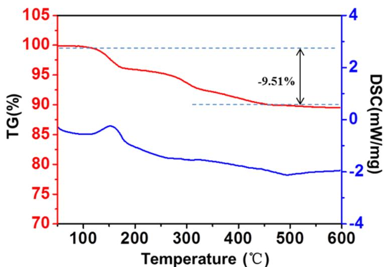
**Figure S2.** TGA-DTA analysis of the pristine  $\text{Mg}_{0.3}\text{V}_2\text{O}_5 \cdot 1.1\text{H}_2\text{O}$ . The  $\text{Mg}_{0.3}\text{V}_2\text{O}_5 \cdot 1.1\text{H}_2\text{O}$  shows stepwise loss of lattice water corresponding to an overall 9.51% weight loss, equivalent to 1.1 molecule of water per formula unit.
