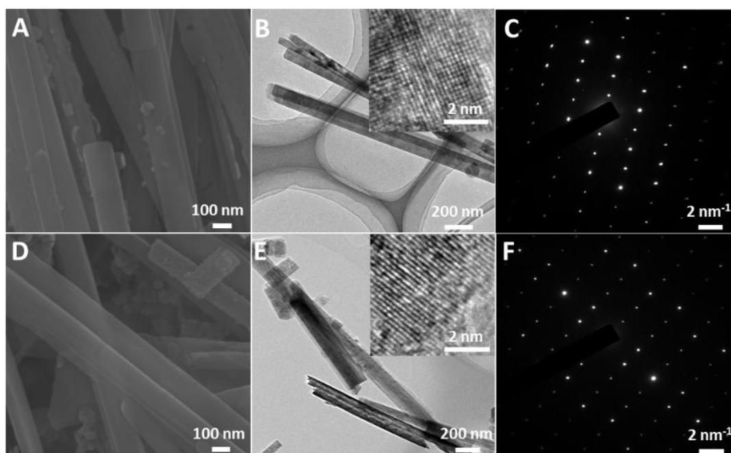
**Figure S12.** (A) SEM image, (B) TEM image, (insets of B) HRTEM image and (C) SAED pattern of  $Mg_{0.3}V_2O_5 \cdot 1.1H_2O$  after 500 cycles at  $0.1 \text{ A g}^{-1}$ . (D) SEM image, (E) TEM image, (insets of E) HRTEM image and (F) SAED pattern of  $Mg_{0.3}V_2O_5 \cdot 1.1H_2O$  after 10000 cycles at  $1 \text{ A g}^{-1}$ .
