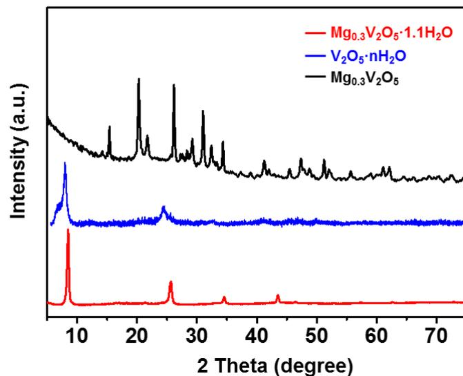
**Figure S1.** XRD diffraction patterns of  $\text{Mg}_{0.3}\text{V}_2\text{O}_5 \cdot 1.1\text{H}_2\text{O}$ ,  $\text{V}_2\text{O}_5 \cdot n\text{H}_2\text{O}$  and  $\text{Mg}_{0.3}\text{V}_2\text{O}_5$ .
