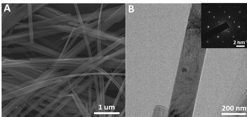
**Figure S5.** (A) FESEM image, (B) TEM images and (inset of B) SAED pattern of  $\text{V}_2\text{O}_5 \cdot n\text{H}_2\text{O}$ .
