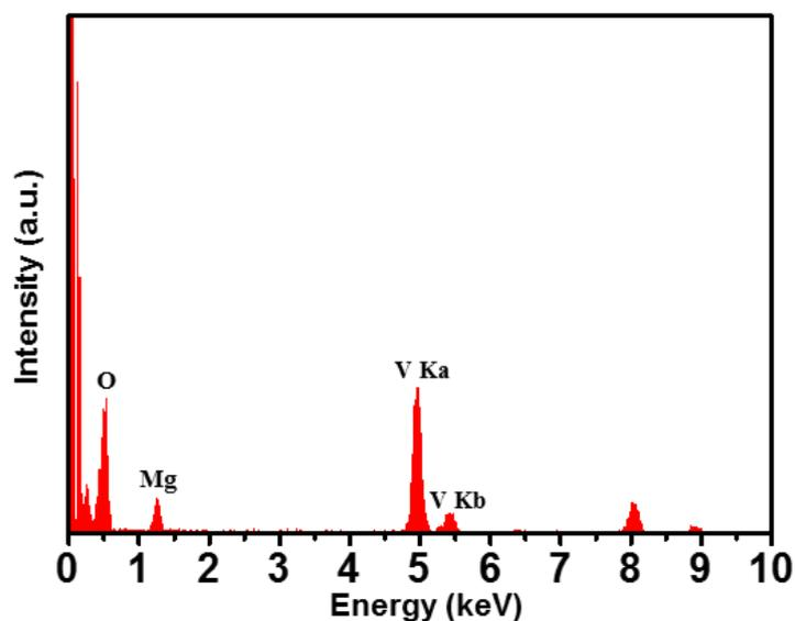
**Figure S18.** EDX spectrum of Mg<sub>0.3</sub>V<sub>2</sub>O<sub>5</sub>·1.1H<sub>2</sub>O cathode in discharging state in MgNaTi<sub>3</sub>O<sub>7</sub>/Mg<sub>0.3</sub>V<sub>2</sub>O<sub>5</sub>·1.1H<sub>2</sub>O full cell.
