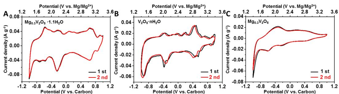
**Figure S8.** CV curves of (A)  $\text{Mg}_{0.3}\text{V}_2\text{O}_5 \cdot 1.1\text{H}_2\text{O}$ , (B)  $\text{V}_2\text{O}_5 \cdot n\text{H}_2\text{O}$  and (C)  $\text{Mg}_{0.3}\text{V}_2\text{O}_5$  for the first two cycle at a scanning rate of  $0.1 \text{ mV s}^{-1}$  between 1.4 and 3.4 V vs.  $\text{Mg}/\text{Mg}^{2+}$ .
