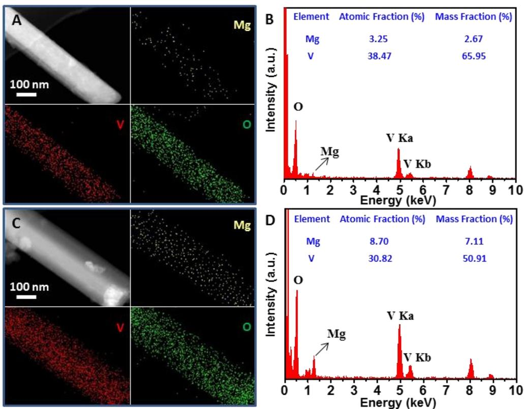
**Figure S13.** (A) TEM-EDX element mapping images of  $\text{Mg}_{0.3}\text{V}_2\text{O}_5 \cdot 1.1\text{H}_2\text{O}$  nanowires at full charge state in 10<sup>th</sup> cycle, and (B) corresponding energy dispersive X-ray (EDX) spectrum. (C) TEM-EDX element mapping images of  $\text{Mg}_{0.3}\text{V}_2\text{O}_5 \cdot 1.1\text{H}_2\text{O}$  nanowires at full discharge state in 10<sup>th</sup> cycle, and (D) corresponding energy dispersive X-ray (EDX) spectrum.
