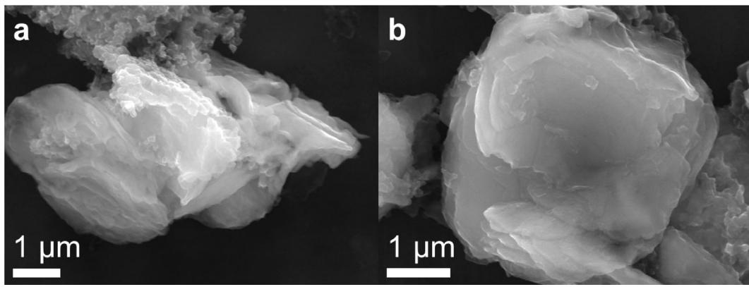
**Figure S8** SEM images of (a) FMO and (b) FMO/GO after 50 cycles in sodium storage.
