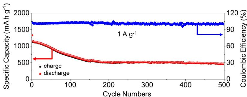
**Figure S5** The long-term cycling performance of FMO/GO at  $1 \text{ A g}^{-1}$  in LIBs.
