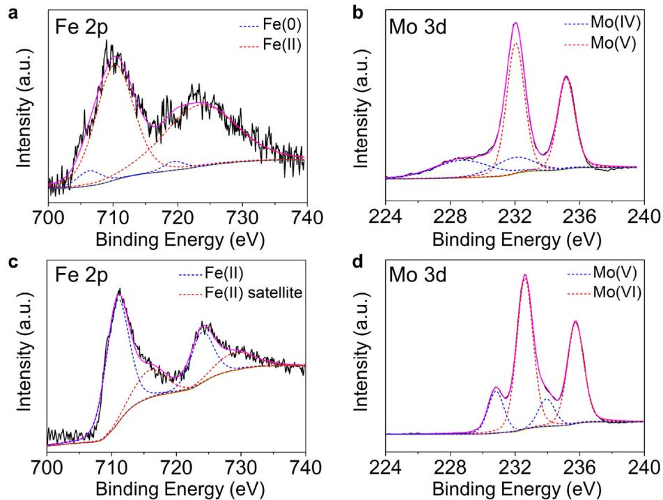
**Figure S9** XPS spectra of FMO when discharged to 0.01 V (a, b) and charged to 3 V (c, d).
