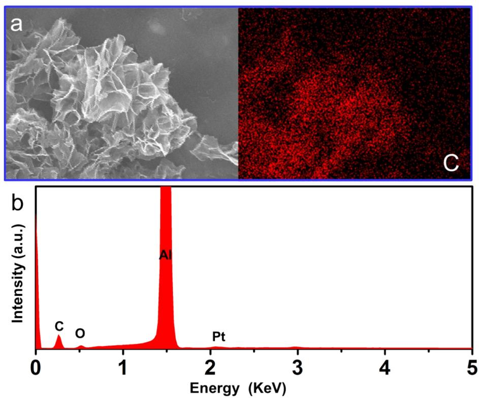
**Fig. S3** (a) EDS elemental mappings, and (b) EDS spectrum of the residual carbon skeleton after etching the LTP from LTP-F/C.
