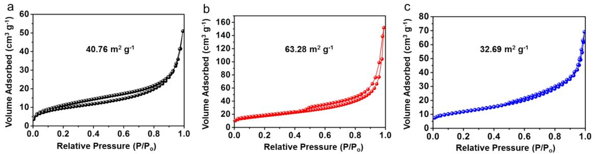
**Fig. S2** Nitrogen adsorption-desorption isotherms of (a) LTP-F precursor, (b) LTP-F/C and (c) bare LTP.
