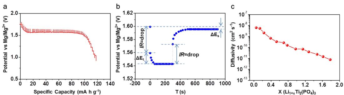
**Fig. S11** (a) GITT curve of LTP-F/C at 1.0-2.0 V, (b) GITT potential response curve with time. The experiment was carried out at constant current pulse of 50 mA g<sup>-1</sup> for 5 min followed by a relaxation period of 10 min and avoltage range.(c) Diffusivity versus state of discharge.
