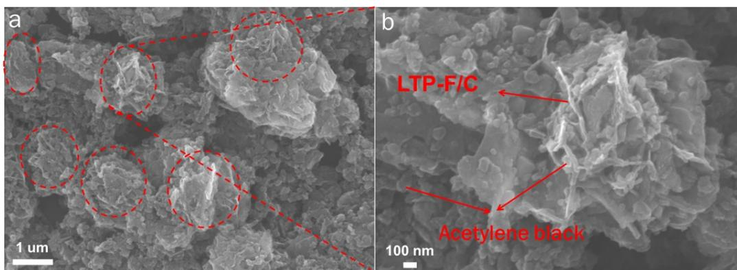
**Fig. S12** (a, b) SEM images of the LTP-F/C electrode after 3000 cycles at 10 C.
