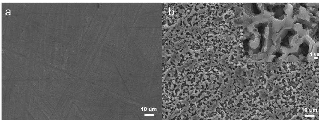
**Fig. S13** SEM images of the Mg anode before cycling (a) and after 3000 cycles at 10 C (b).
