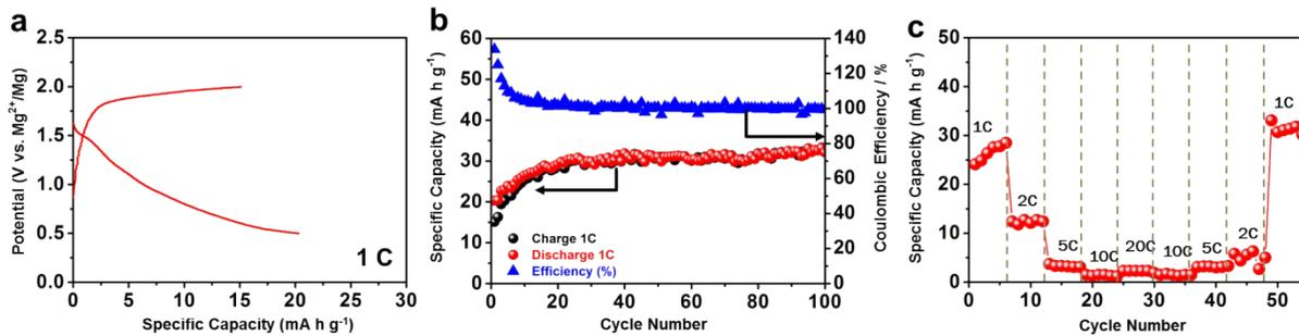
Fig. S6 (a) The initial discharge-charge curves and (b) cycling performances of bare LTP at 1 C. (c) The rate performances of bare LTP.
