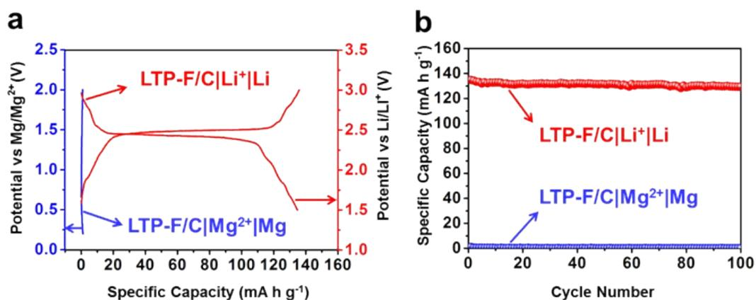
**Fig. S10** (a) Discharge/charge curves of LTP-F/C cathode in the LTP-F/C|Mg<sup>2+</sup>|Mg cell (1st cycle), LTP-F/C|Li<sup>+</sup>|Li cell (1st cycle), at 1 C (  $1 \text{ C} = 140 \text{ mA h g}^{-1}$  ) and (b) corresponding cycling performances.
