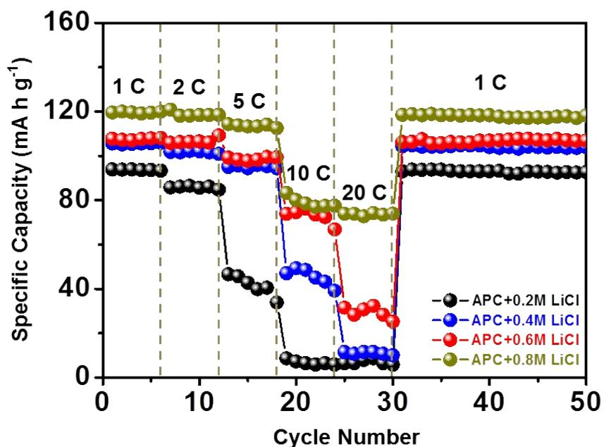
**Fig. S8** Rate performances of LTP-F/C under different concentrations of LiCl.
