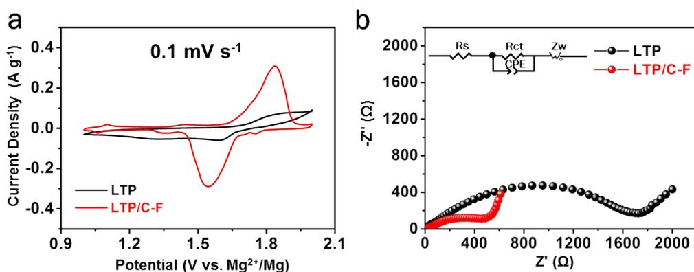
**Fig. S9** (a) CV curves of LTP-F/C and bare LTP for the first cycle at a scanning rate of  $0.1 \text{ mV s}^{-1}$ . (b) The Nyquist plots of the LTP-F/C and bare LTP after two cycles with equivalent circuit inset.
