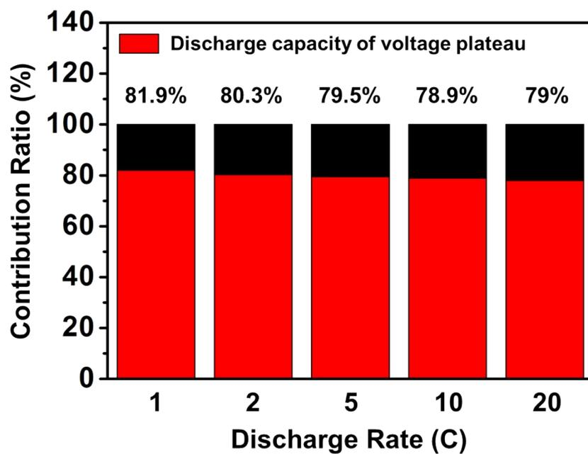
Fig. S7 Contribution ratio of plateau discharge capacity of LTP-F/C at different rates.
