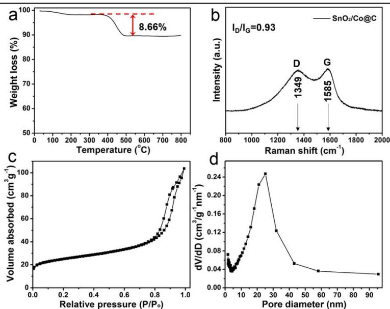
**Figure S5.** (a) TGA curve, (b) Raman spectrum, (c, d) N<sub>2</sub> adsorption/desorption isotherm and the corresponding pore size distribution of SnO<sub>2</sub>/Co@C nanocubes.
