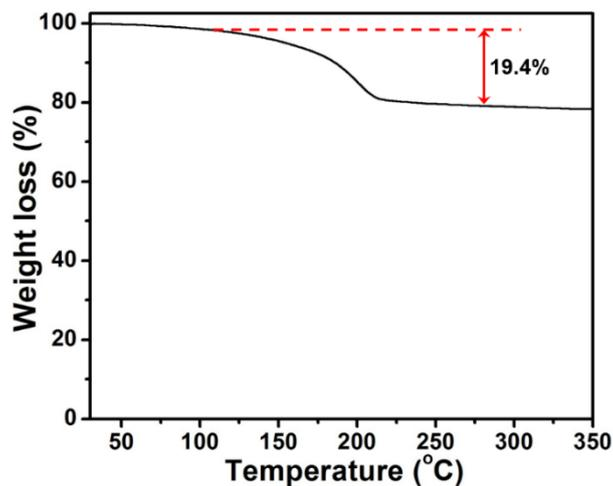
**Figure S2.** TGA curve of  $\text{CoSn(OH)}_6$  which was tested in air from 30 °C to 350 °C with the temperature rising rate of 2 °C  $\text{min}^{-1}$ .
