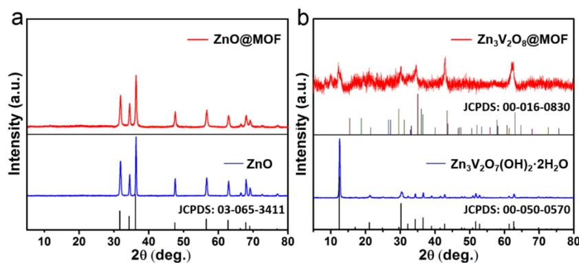
**Figure S6.** XRD patterns of (a) ZnO and ZnO@MOF microflowers, (b) Zn<sub>3</sub>V<sub>2</sub>O<sub>7</sub>(OH)<sub>2</sub>·2H<sub>2</sub>O and Zn<sub>3</sub>V<sub>2</sub>O<sub>8</sub>@MOF nanoplates, respectively.
