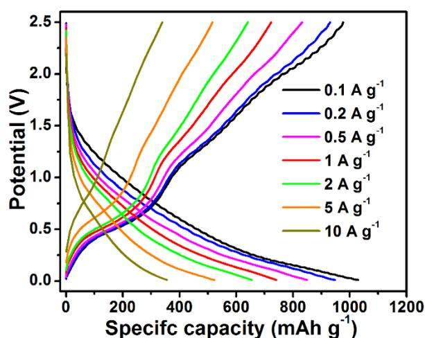
**Figure S7.** The charge-discharge voltage profiles of the SnO<sub>2</sub>/Co@C nanocubes at different current densities.
