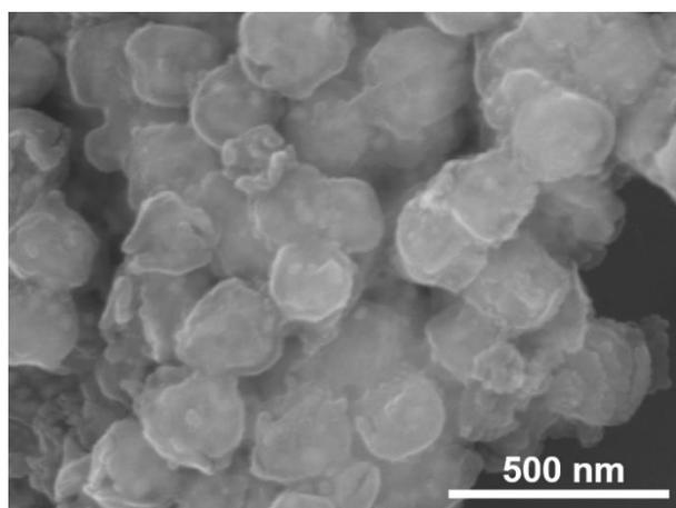
**Figure S9.** SEM image of SnO<sub>2</sub>/Co@C nanocubes after cycling for 100 cycles under the current density of 200 mA g<sup>-1</sup> within the potential range of 0.01~2.5 V.
