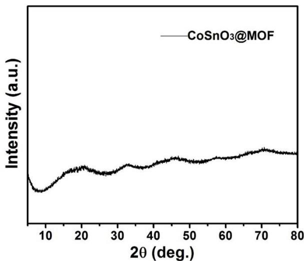
**Figure S3.** XRD pattern of the hollow  $\text{CoSnO}_3@MOF$  nanocubes.
