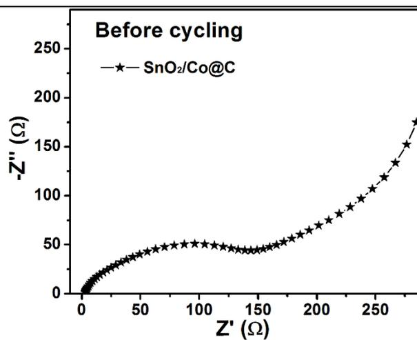
**Figure S8.** Nyquist plot of the SnO<sub>2</sub>/Co@C nanocubes electrode.
