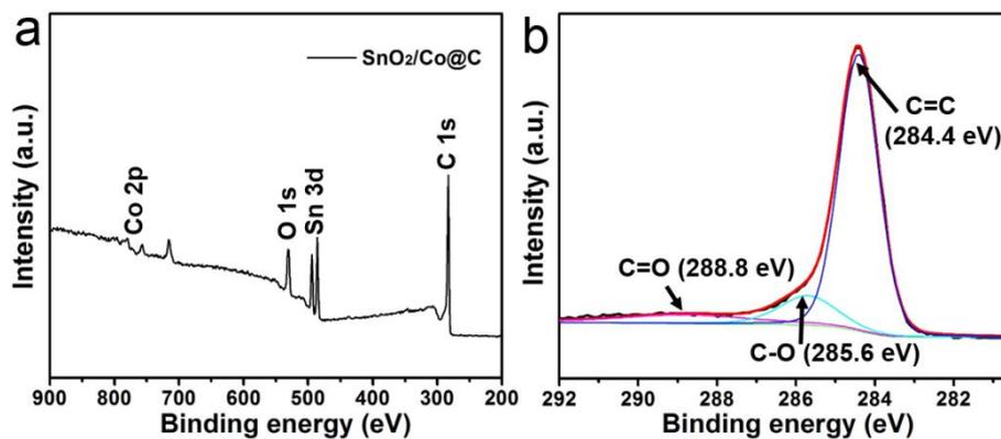
**Figure S4.** (a) XPS spectrum for survey scans of  $\text{SnO}_2/\text{Co}@C$  nanocubes and (b) corresponding C 1s core-level spectrum.
