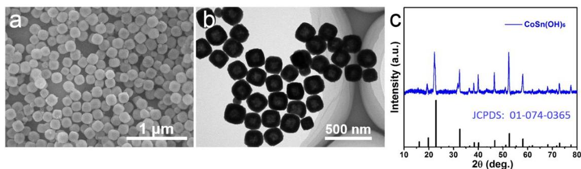
**Figure S1.** (a) SEM image, (b) TEM image, (c) XRD pattern of hollow  $CoSn(OH)_6$  nanocubes.
