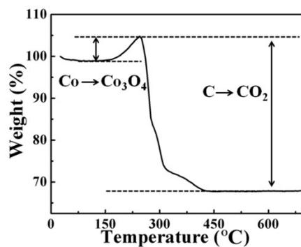
**Figure S7.** TG curve of Co/NPCNW between 0 and 700 °C measured with a heating rate of 5 °C min<sup>-1</sup> under air atmosphere.
