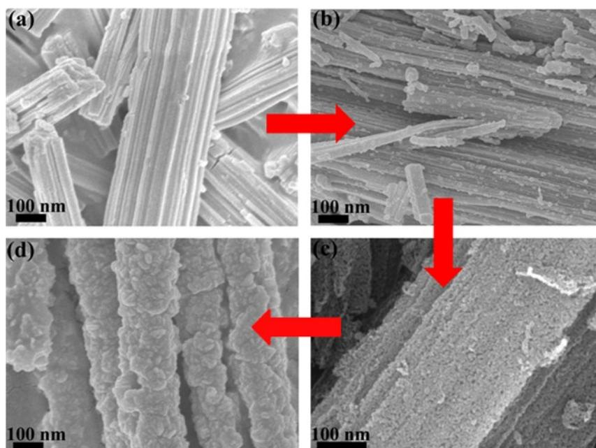
**Figure S5.** SEM images of the Co-MOF (a) and the calcined samples for 1 h (b), 2 h (c), 3 h (d) at 700 °C.
