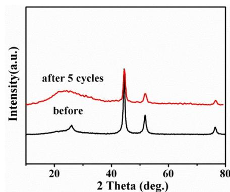
**Figure S15.** XRD patterns of the Co/NPCNW before and after 5 cycles.
