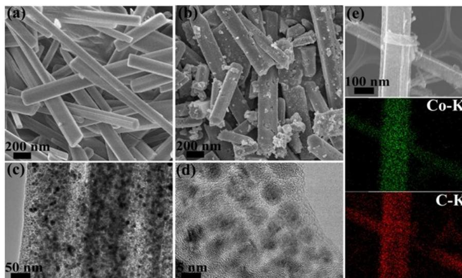
**Figure S9.** SEM images of Co-MOF (the precursor of Co/C) (a) and Co/C (b); TEM (c), HRTEM images (d), and SEM mapping (e) of Co/C.
