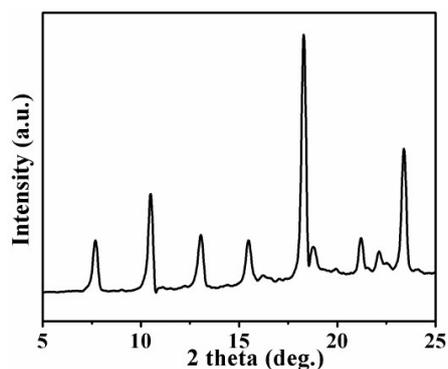
Figure S1. XRD pattern of the as-prepared Co-MOF.
