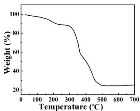
Figure S3. TG curve of Co/NPCNW between 0 and 700 °C measured with a heating rate of 5 °C min<sup>-1</sup> under Ar atmosphere.
