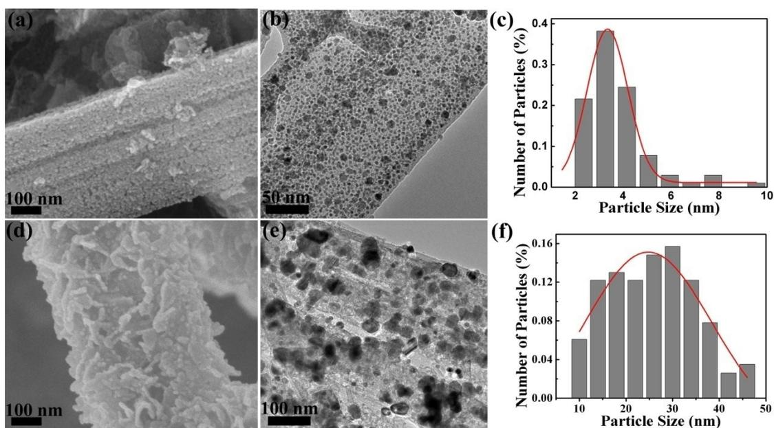
**Figure S6.** SEM and TEM images of the calcined Co-MOF for 2 h (a, b) and 3 h (d, e) at 700 °C and the corresponding size distribution of cobalt nanoparticles (e, 2 h; f, 3 h).
