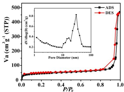
Figure S2. N<sub>2</sub> adsorption-desorption isotherm of the as-prepared Co-MOF (inset is the pore-size distribution of Co-MOF).
