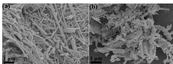
Figure S4. SEM images of the calcined Co-MOF with the calcination temperature at 700 °C (a) and 800 °C (b) for 2 h.
