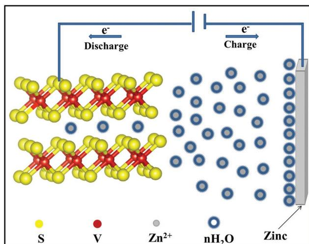
**Figure 4.** Schematic illustration of the operation mechanism of Zn/VS<sub>2</sub> batteries
