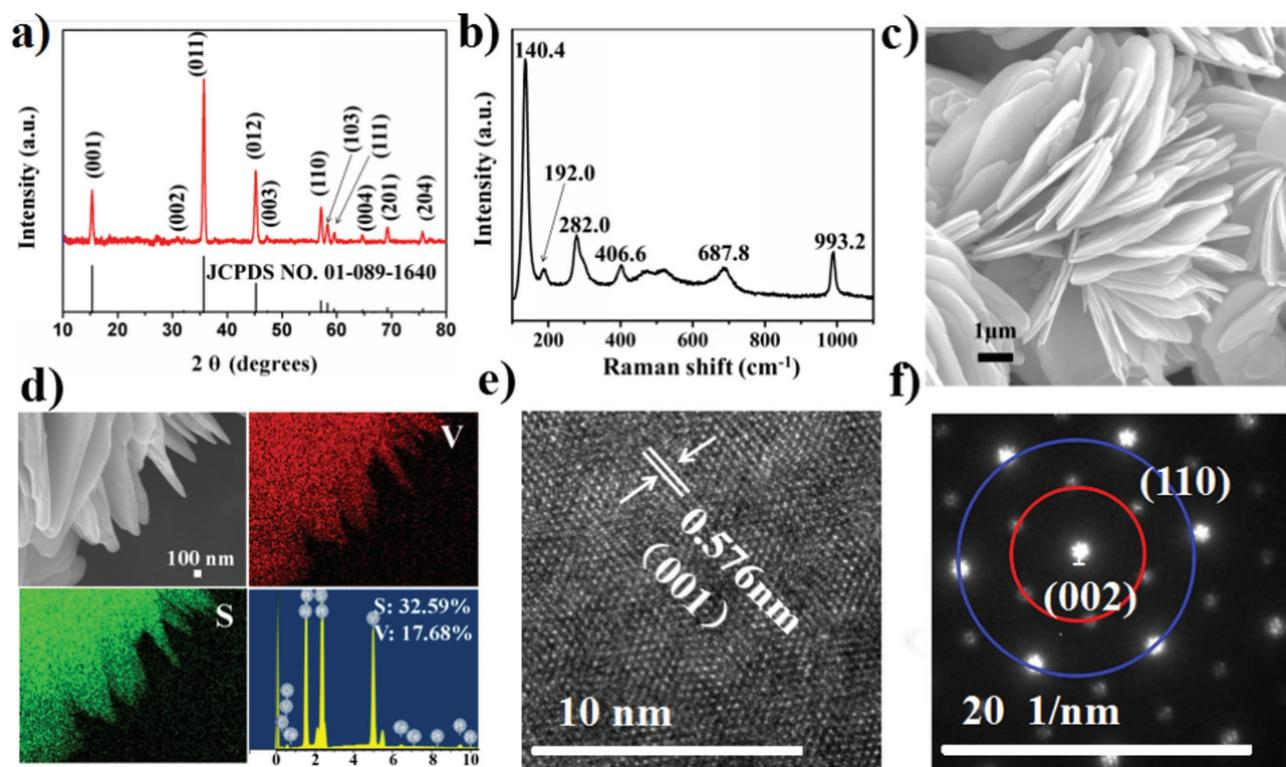
**Figure 1.** The characterization of layered  $\text{VS}_2$ : a) XRD pattern, b) Raman spectra, c) SEM, d) SEM-EDX, e) HR-TEM image, and f) SAED.
