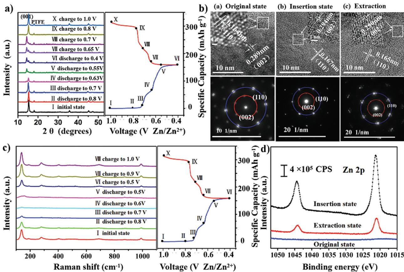
**Figure 3.** a) Ex situ XRD patterns of VS<sub>2</sub> collected at various states. b) HR-TEM images and SAED patterns. c) In situ Raman spectra of VS<sub>2</sub> electrode at a scan rate of 2.0 mV s<sup>-1</sup> in the voltage range of 0.4–1.0 V. d) Zn 2p core level spectra of VS<sub>2</sub> electrodes in original, insertion, and extraction states.
