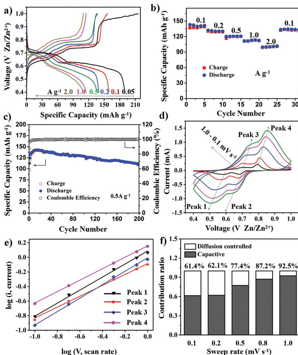
**Figure 2.** Electrochemical performances of Zn/VS<sub>2</sub> batteries cycling in a range of 0.4–1.0 V. a) Charge and discharge curves at the current density from 0.05 to 2.0 A g<sup>-1</sup>. b) Rate capability. c) Long-term cyclic properties at a current density of 0.5 A g<sup>-1</sup>. d) CV curves at different scan rates. e) Log(*i*) versus log(*v*) plots at specific peak currents. f) The contribution ratio of the capacitive capacities and diffusion-limited capacities.
