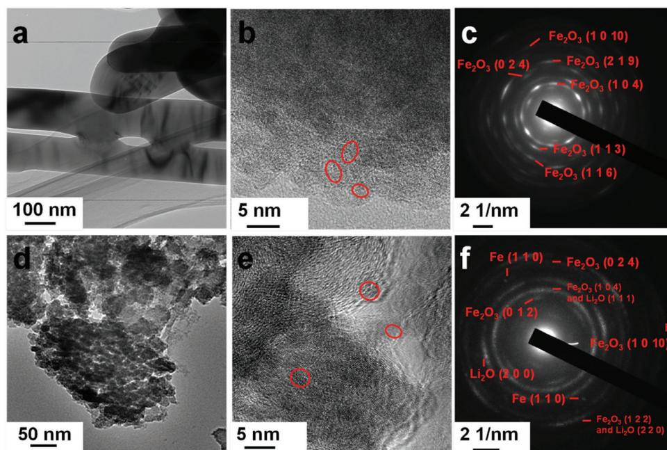
**Figure 4.** a,b) TEM images of  $\alpha$ -Fe<sub>2</sub>O<sub>3</sub>-800 after ten cycles. c) The corresponding SAED pattern of  $\alpha$ -Fe<sub>2</sub>O<sub>3</sub>-800 after ten cycles. d,e) TEM images of  $\alpha$ -Fe<sub>2</sub>O<sub>3</sub>-500 after ten cycles. f) The corresponding SAED pattern of  $\alpha$ -Fe<sub>2</sub>O<sub>3</sub>-500 after ten cycles.
