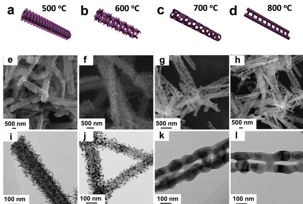
**Figure 2.** Schematic illustrations, SEM images, and TEM images of a,e,i)  $\alpha$ -Fe<sub>2</sub>O<sub>3</sub>-500, b,f,j)  $\alpha$ -Fe<sub>2</sub>O<sub>3</sub>-600, c,g,k)  $\alpha$ -Fe<sub>2</sub>O<sub>3</sub>-700, and d,h,l)  $\alpha$ -Fe<sub>2</sub>O<sub>3</sub>-800.
