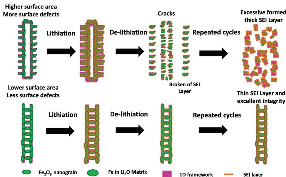
Figure 5. Schematic illustration of morphology evolution and SEI formation of  $\alpha$ -Fe<sub>2</sub>O<sub>3</sub>-800 and  $\alpha$ -Fe<sub>2</sub>O<sub>3</sub>-500 during discharge/charge cycling.
