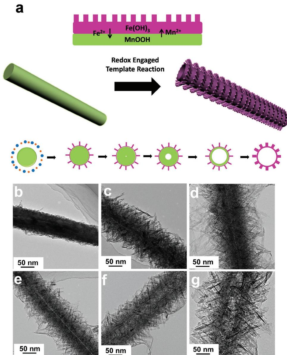
**Figure 1.** a) Schematic illustrations of the formation process. b–g) TEM images of the products with different reaction durations: 10 min (b), 30 min (c), 1 h (d), 2 h (e), 6 h (f), and 12 h (g), respectively.
