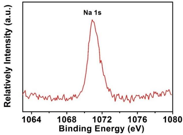
**Fig. S5** High-resolution XPS spectrum of Na 1s of the  $\text{H}_2\text{V}_3\text{O}_8$  nanowire membrane discharged to 1.5 V.
