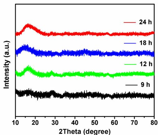
**Figure S2.** XRD patterns of carbon-supported and nanosheets-assembled amorphous vanadium oxide microspheres prepared at 9, 12, 18 and 24 h, respectively.
