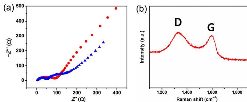
**Figure S4** (a) AC impedance plots of amorphous vanadium oxide microspheres (red) and crystalline  $V_2O_3$  microspheres (blue), respectively. (b) Raman spectra of crystalline  $V_2O_3$  microspheres.
