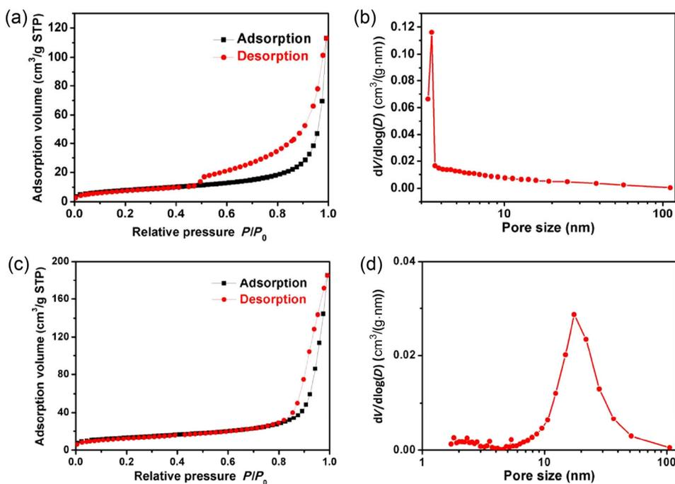
**Figure S6** (a) and (b) Nitrogen adsorption-desorption isotherms and the corresponding pore size distribution of amorphous vanadium oxide microspheres; (c) and (d) nitrogen adsorption-desorption isotherms and the corresponding pore size distribution of crystalline  $V_2O_3$  microspheres.
