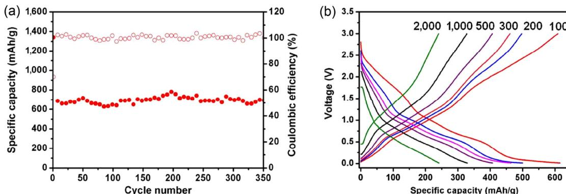
**Figure S7** (a) Cycling performance and Coulombic efficiency of amorphous vanadium oxide microspheres tested at 100 mA/g. (b) Charge-discharge curves of amorphous vanadium oxide microspheres tested at different current densities ranging from 100 to 200, 300, 500, 1,000, 2,000 mA/g, respectively.
