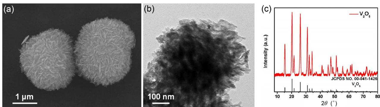
**Figure S1** SEM image (a), TEM image (b) and XRD pattern (c) of V<sub>2</sub>O<sub>5</sub> microspheres assembled with nanosheets, which is obtained after sintering in air.
