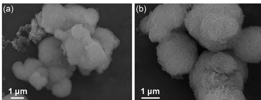
**Figure S8** SEM images of amorphous vanadium oxide microspheres (a) and crystalline  $V_2O_3$  microspheres (b) after cycling 400 times at the current density of 200 mA/g.
