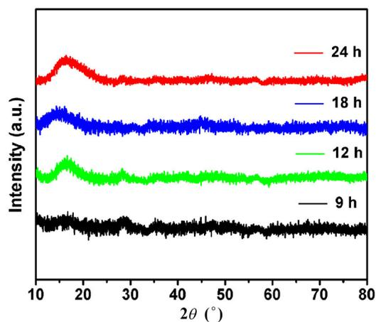
**Figure S2** XRD patterns of carbon-supported and nanosheet-assembled amorphous vanadium oxide microspheres prepared at 9, 12, 18 and 24 h, respectively.
