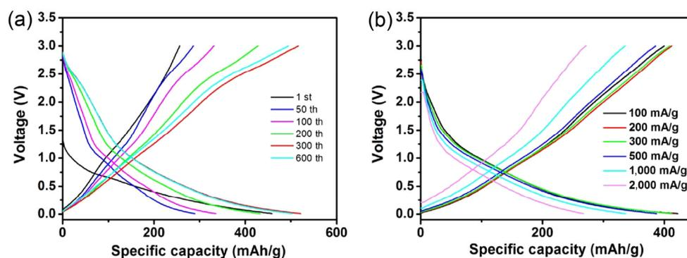
**Figure S9** (a) The voltage profiles of crystalline  $V_2O_3$  microspheres tested at the current density of 200 mA/g. (b) The charge and discharge curves of crystalline  $V_2O_3$  microspheres tested at different current densities ranging from 100 to 2,000 mA/g.
