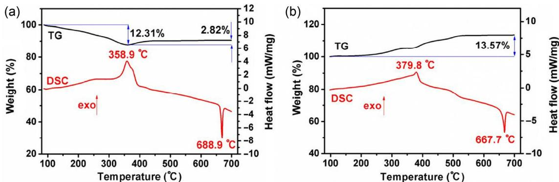
**Figure S5** TG (black line) and DSC (red line) of amorphous vanadium oxide microspheres (a) and crystalline  $V_2O_3$  microspheres (b), respectively.
