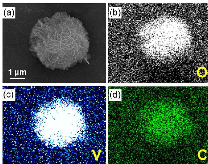
**Figure S3** SEM image (a) and EDS elemental mappings of carbon-supported and nanosheet-assembled amorphous vanadium oxide microspheres. The elements of oxygen (b), vanadium (c), and carbon (d) are characterized, respectively.
