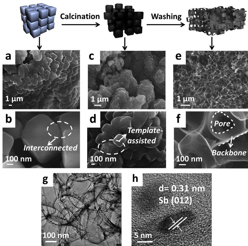
**Fig. 3.** SEM & TEM characterization and schematic illustration of the samples at different states. (a, b) SEM images of the  $\text{SbCl}_3$ /citric acid/PVP/NaCl composite particles after freeze-drying; (c, d) SEM images of  $\text{SbNPs}@3\text{D-C}@NaCl$ ; (e, f) SEM images of  $\text{SbNPs}@3\text{D-C}$ ; (g) TEM image of  $\text{SbNPs}@3\text{D-C}$ ; (h) HRTEM image of  $\text{SbNPs}@3\text{D-C}$ .
