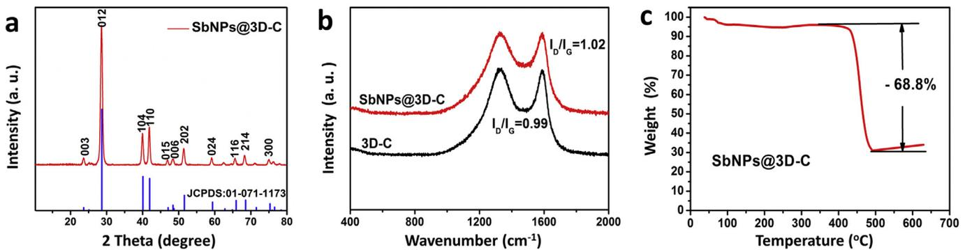
Fig. 2. (a) XRD pattern of the SbNPs@3D-C. (b) Raman spectra of the SbNPs@3D-C and 3D-C. (c) TGA profile of the SbNPs@3D-C.
