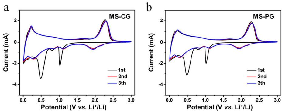
**Figure S4.** CV curves of the first three cycles of the MS-CG (a) and the MS-PG (b).
