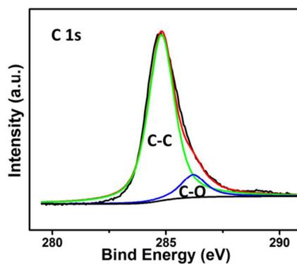
**Figure S3.** The high resolution C 1s spectrum of MS-CG.
