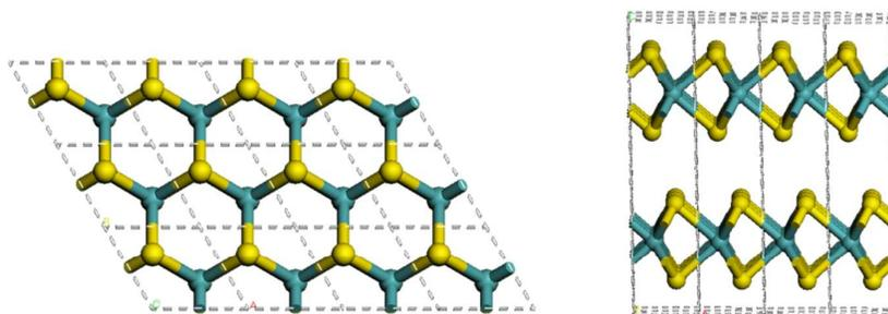
**Figure S2.** Stick and ball lattice structure of the hexagonal 2H phase  $MoS_2$ . Blue and yellow spheres represent molybdenum (Mo) and surplus (S) atoms, respectively. In detail, the S atoms in the lattice adopt a hexagonal close-packing structure. The Mo atoms are sandwiched between two atomic layers of S, and each Mo is coordinated with six S atoms.
