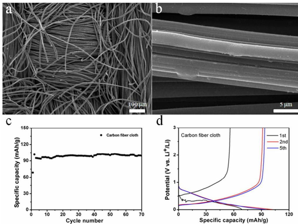
**Figure S6.** (a, b) FESEM images of bare carbon fiber cloth. (c) Cycling performance and (d) charge/discharge profiles of bare carbon fiber cloth at a current density of 100 mA/g.
