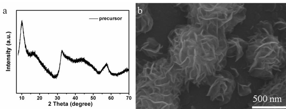
**Figure S1.** (a) XRD pattern and (b) FESEM image of the MS precursor without heat treatment under  $H_2/Ar$  (5%/95%).
