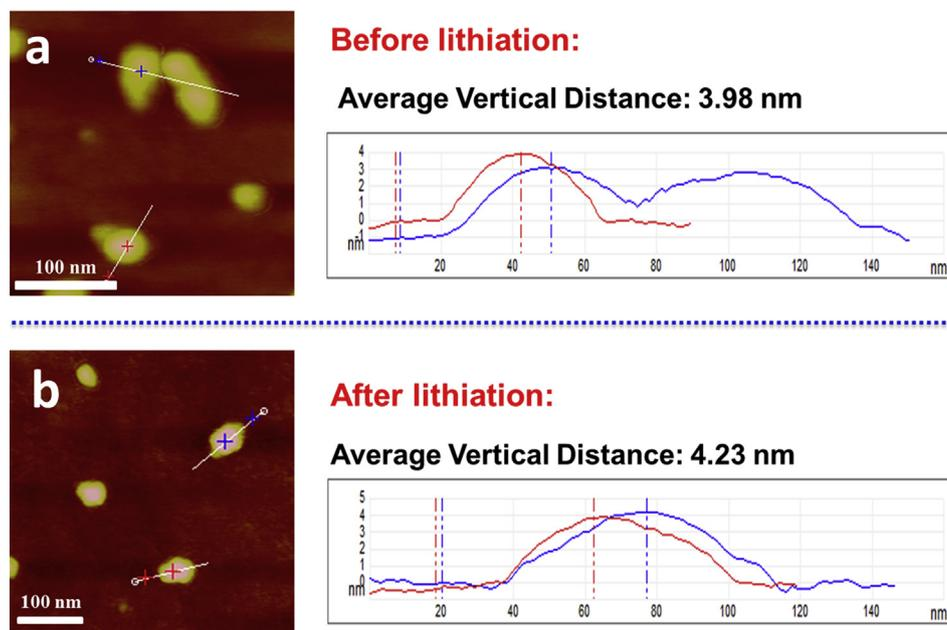
Fig. 2. The AFM images and height profiles of as-prepared (a) ultrathin non-lithiated  $V_6O_{13}$  nanosheets and (b) ultrathin lithiated  $V_6O_{13}$  nanosheets.
