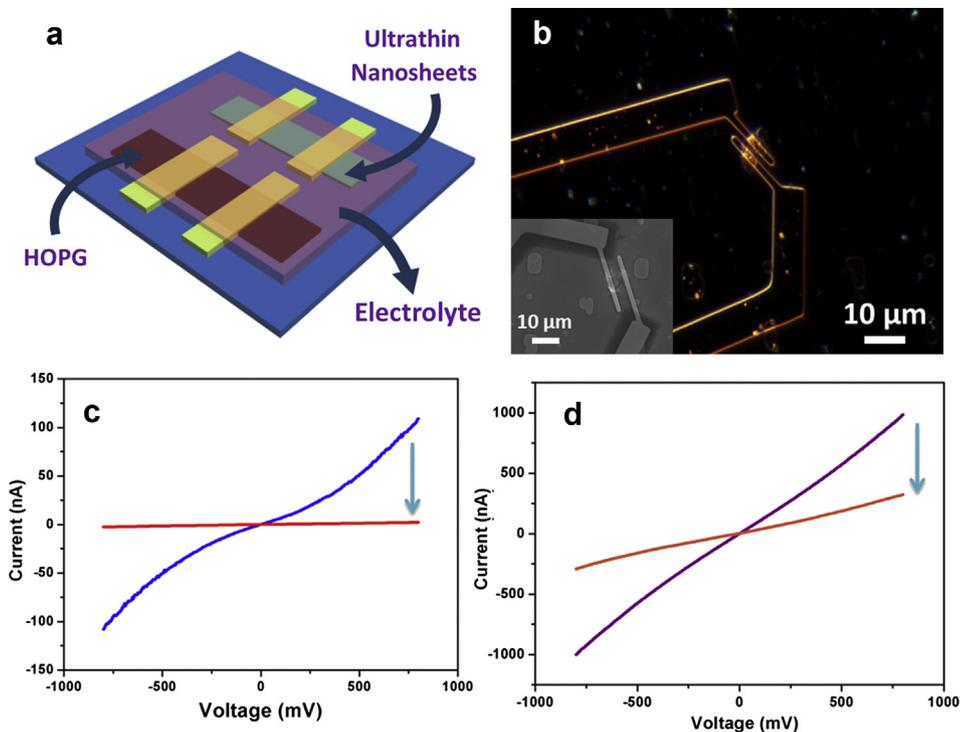
**Fig. 3.** (a) Schematic illustration of assembled nanosheet cathodes based energy storage device. (b) The dark-field optical microscopy image of nanosheets cathode before  $\text{Li}^+$  intercalation. Inset shows the SEM image of nanosheets cathode after  $\text{Li}^+$  intercalation. (c, d) The transport properties of non-lithiated (c) and pre-lithiated nanosheets cathode (d) before and after  $\text{Li}^+$  intercalation.
