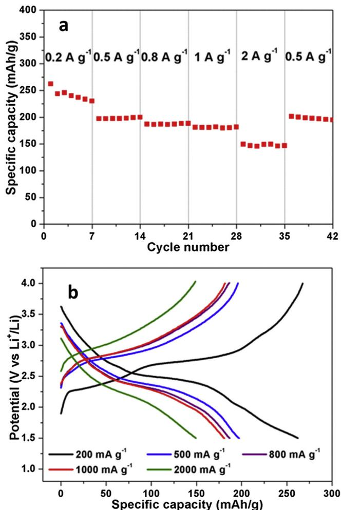
Fig. 5. (a) Rate performance and (b) initial charge–discharge curves of ultrathin lithiated  $\text{V}_6\text{O}_{13}$  nanosheets at various current densities from 200 to  $2000 \text{ mA g}^{-1}$ .
