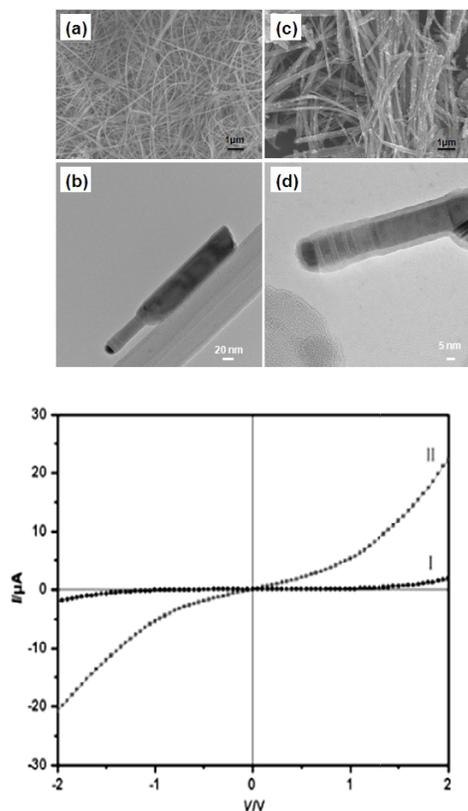
**Figure 3.** (a, b) Typical FE-SEM and TEM images of  $\beta$ -AgVO<sub>3</sub> nanowires. (c, d) Typical FE-SEM and TEM images of AgVO<sub>3</sub>/PPy nanocables. (e) I-V curves of  $\beta$ -AgVO<sub>3</sub> nanowires (I) and AgVO<sub>3</sub>/PPy nanocables(II).
