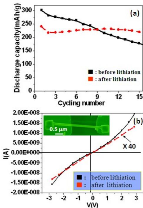
**Figure 4.** (a) The discharge capacity as a function of the cycle number for the MoO<sub>3</sub> nanowires before and after lithiation. (b) I/V transport measurements of single nanowire fabricated devices using the samples before and after lithiation [16].
