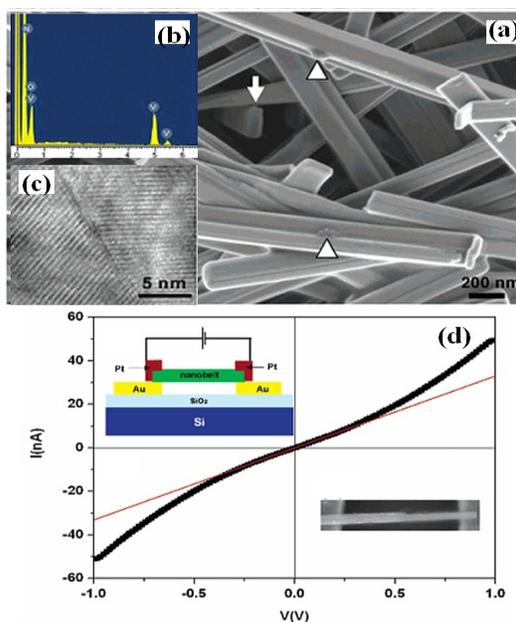
**Figure 1.** (a, b) Scanning electron microscope (SEM) image and energy dispersive spectroscopy (EDS) spectrum of  $\text{NH}_4\text{V}_3\text{O}_8$  nanowire. (c) The representative high-resolution transmission electron microscope (HRTEM) image of the twin boundary present in a nanowire. (d) Current-voltage ( $I/V$ ) curve of individual nanowire. Insets: the schematic view and the SEM image of the individual nanowire electrode, respectively [23].
