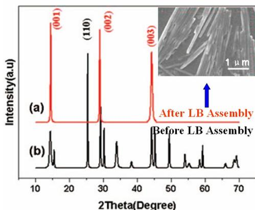
**Figure 5.** The X-ray diffraction (XRD) patterns of VO<sub>2</sub> nanowire LB films (a) and as-synthesized VO<sub>2</sub> nanowires without LB assembly (b). The inset is the SEM image of VO<sub>2</sub> nanowire LB films [53].
