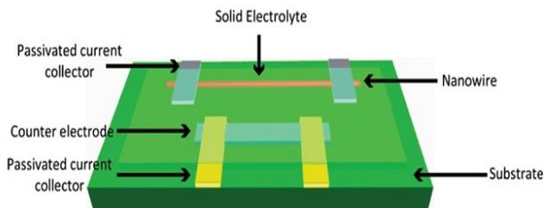
**Figure 2.** Schematic diagram of a single nanowire electrode device design [9].
