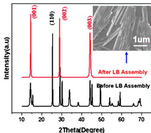
FIG. 3. XRD patterns of  $\text{VO}_2$  nanowires before and after Langmuir-Blodgett (LB) assembly. Insert is the SEM image of  $\text{VO}_2$  nanowire LB film.<sup>31</sup>
