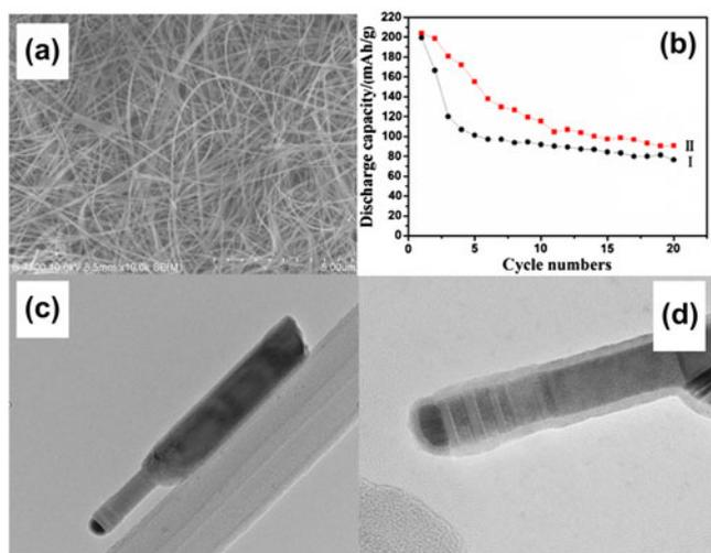
FIG. 6. (a) Typical FESEM image of the  $\beta$ -AgVO<sub>3</sub> nanowires. (b) Cyclability of the batteries assembled with the  $\beta$ -AgVO<sub>3</sub> nanowires (I) and the AgVO<sub>3</sub>-PPy nanocables (II). (c) and (d) Typical TEM images of AgVO<sub>3</sub> and AgVO<sub>3</sub>/PPy nanocable, respectively.<sup>54</sup>
