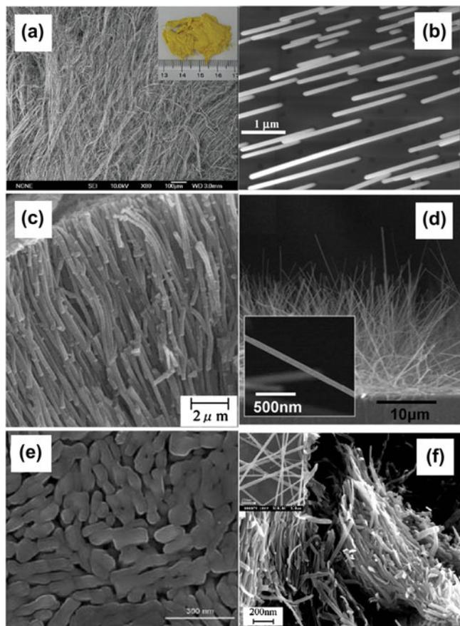
FIG. 1. Scanning electron microscope (SEM) images of vanadium oxide nanowires or nanorods synthesized by different methods. (a) Hydrothermal.<sup>15</sup> (b) CVD.<sup>16</sup> (c) Template assisted.<sup>17</sup> (d) Vapor transport.<sup>20</sup> (e) Thermal decomposition.<sup>21</sup> (f) Electrospinning combined with hydrothermal.<sup>25</sup>
