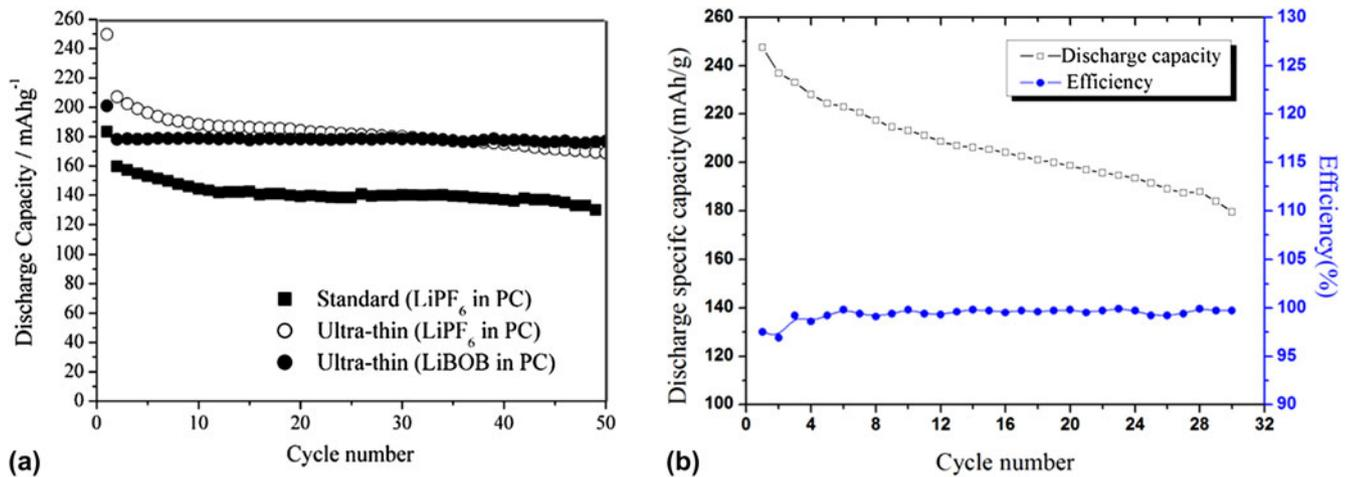
FIG. 4. (a) Discharge capacity versus cycle number for  $VO_2(B)$  nanowires in  $LiPF_6$  and lithium bis(oxalate)borate (LiBOB).<sup>37</sup> (b) Discharge specific capacity and efficiency versus cycling number for  $VO_2(B)$  nanowires.<sup>38</sup>
