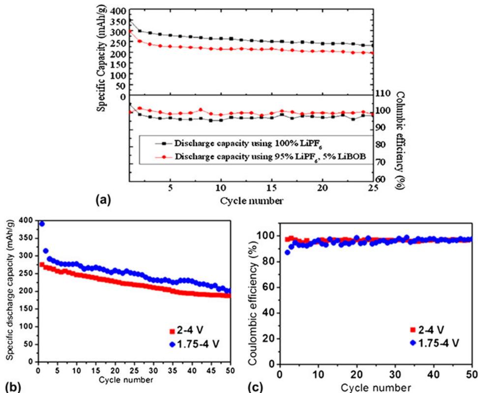
FIG. 5. (a) Capacity and cycling efficiency versus cycle number of nano- $V_2O_5$  using a pure  $LiPF_6$  electrolyte solution and one containing 5% LiBOB.<sup>25</sup> (b) and (c) Capacity versus cycle number and coulombic efficiency versus cycle number of the ultralong hierarchical vanadium oxide nanowires.<sup>28</sup>
