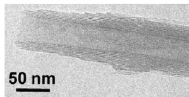
Fig. 3. TEM pattern of vanadium oxide nanotubes.
