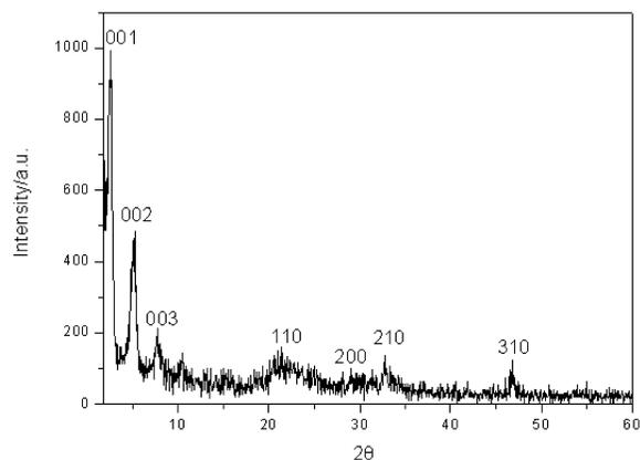
Fig. 1. XRD pattern of vanadium oxide nanotubes.
