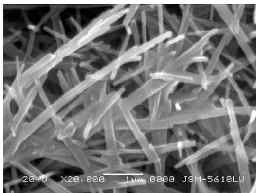
Fig. 2. SEM pattern of vanadium oxide nanotubes.
