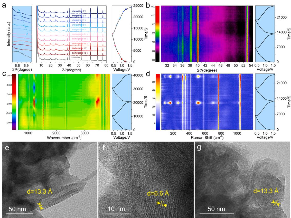
**Fig. 4.** (a) *Ex-situ* and (b) *in-situ* XRD patterns, (c) *in-situ* FTIR spectra, (d) *in-situ* Raman spectra of HAVO-11.0 electrode. *Ex-situ* HRTEM images of HAVO-11.0 electrode (e) in pristine, (f) fully discharged and (g) charged states.
