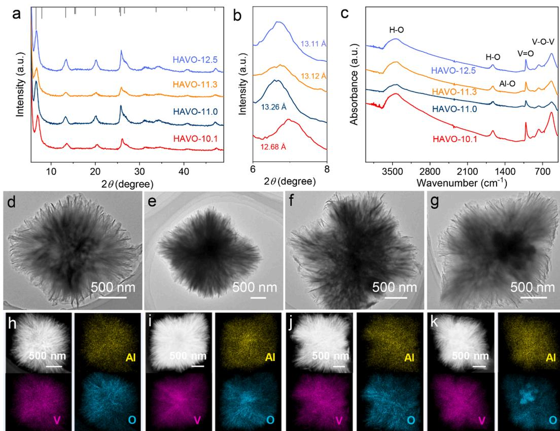
**Fig. 1.** (a) Powder XRD patterns, (b) enlargement of selected regions, and (c) FTIR spectra of HAVOs. (d) TEM image of HAVO-10.1, (h) HAADF-STEM image and corresponding Al, V, O element mapping. (e) TEM image of HAVO-11.0, (i) HAADF-STEM image and EDS mapping image. (f) TEM image, (j) HAADF-STEM image and EDS mapping image of HAVO-11.3. (g) TEM image of HAVO-12.5, (k) HAADF-STEM image and EDS mapping image.
