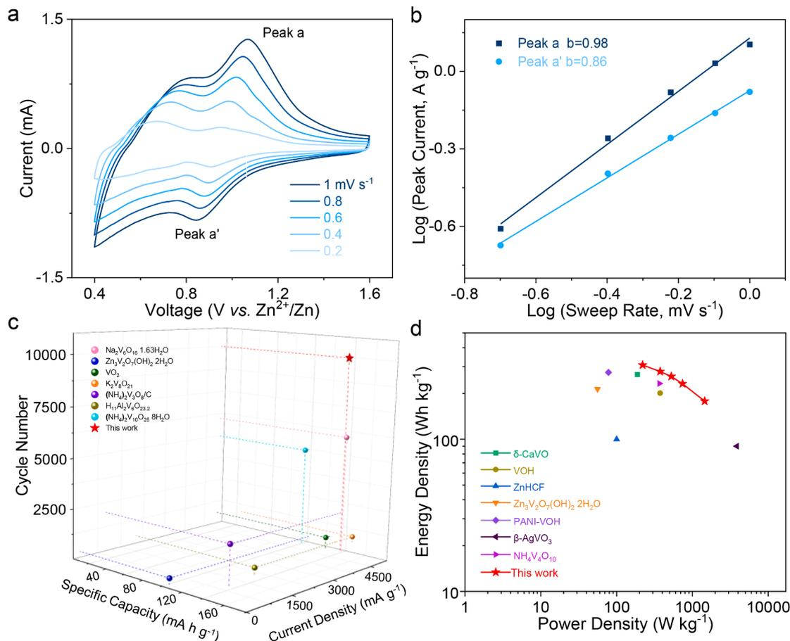
**Fig. 3.** (a) CV curves of HAVO-11.0 at different scan rates. (b) The plots of  $\log$  (peak current) versus  $\log$  (sweep rate) at each peak from CV curves of HAVO-11.0. (c) Comparison of cycling performance with other V-based cathodes. (d) Ragone plots of HAVO-11.0 and other representative cathode materials for AZIBs.
