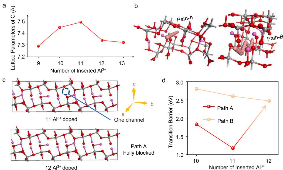
**Fig. 5.** (a) Relationship between the amount of Al<sup>3+</sup> and the lattice parameter of c. (b, c) Sketch map of the two migration paths of Zn<sup>2+</sup> in the cathode. (d) Migration barrier of the Zn<sup>2+</sup> in two paths individually.
