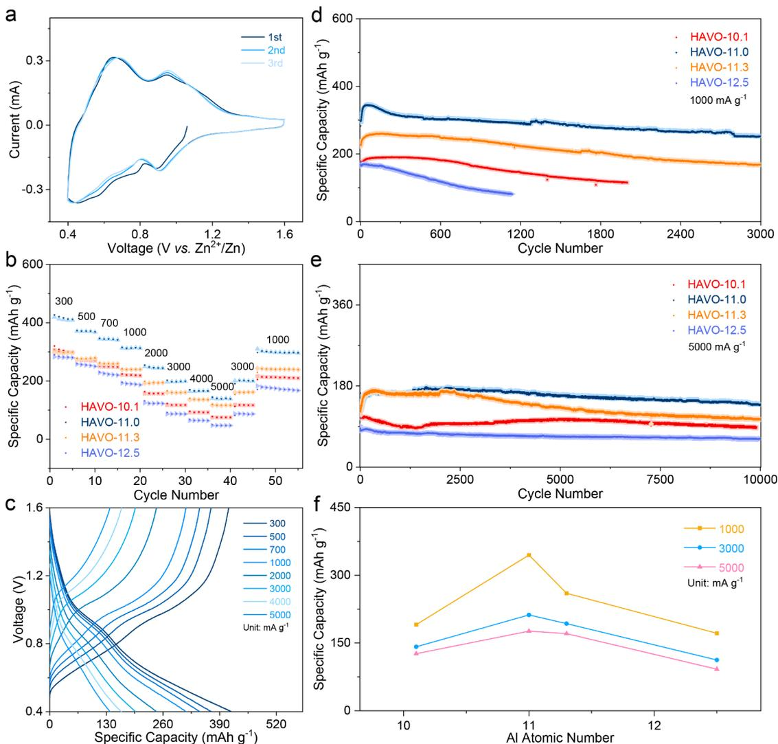
**Fig. 2.** (a) The first three CV curves of HAVO-11.0. (b) Rate capabilities of HAVOs. (c) Charge-discharge curves of HAVO-11.0. Cycling performances tested of HAVOs at (d) 1000 and (e)  $5000\text{ mA g}^{-1}$ . (f) A comparison of the capacitive contribution at different Al atomic numbers of HAVOs.
