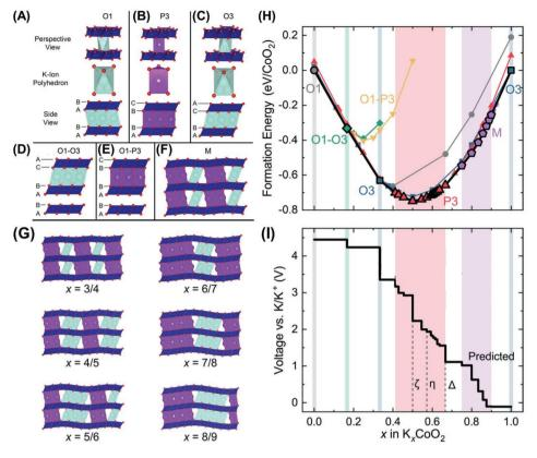
**Figure 6.** Side views show the stacking sequences of the O layers in A) O1, B) P3, C) O3, D) O1–O3, E) O1–P3, F) M, and G) relaxed M ground state structures at select compositions for  $K_x$ CoO<sub>2</sub> host structures. H) Calculated zero-temperature phase diagram and I) predicted voltage curve derived from the zero-temperature formation energies of  $K_x$ CoO<sub>2</sub> for  $0 \le x \le 1$ . Reproduced with permission.<sup>[77]</sup> Copyright 2019, American Chemical Society.
