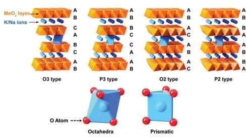
Figure 2. Schematic illustrations of the crystal structures of O3-, P3-, O2-, and P2-A<sub>1-x</sub>MeO<sub>2</sub> (A = K, Na).
