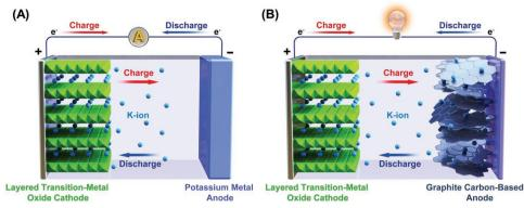
Figure 1. Schematic illustration of the cell configuration and operational mechanism of typical A) half and B) full PIBs.
