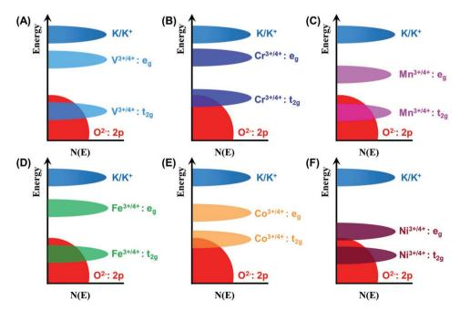
Figure 4. A–F) Schematic diagram of the redox energies of the  $M^{3+/4+}$  couple in K<sub>x</sub>MO<sub>2</sub> (M = V, Cr, Mn, Fe, Co, Ni).
