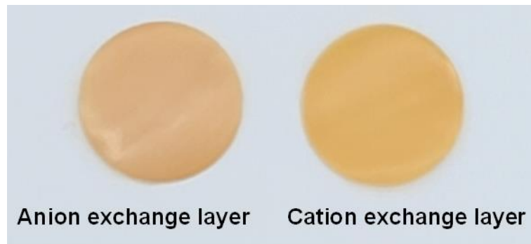
Figure S3. Optical image of the front and back of the bipolar membrane.
