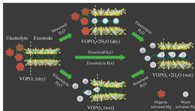
**Fig. 15** Schematic of the solvated  $\text{Mg}^{2+}$  storage mechanisms in  $\text{VOPO}_4 \cdot n\text{H}_2\text{O}$  in dry and wet electrolytes (green curves: activation energy barriers; white dashed lines: electrolyte/electrode interface). Reproduced from ref. 120, with permission from the American Chemical Society.
