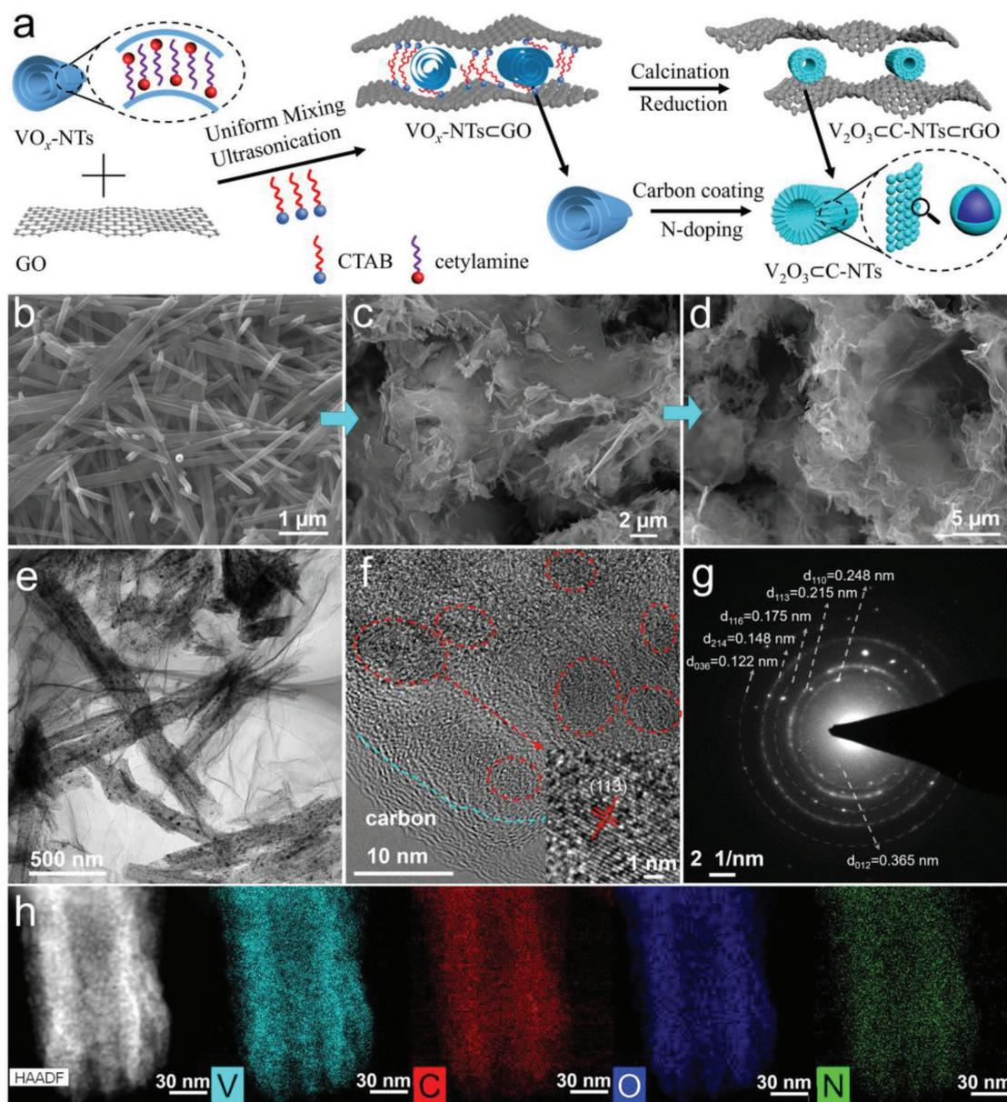
**Figure 2.** Synthesis and characterization of  $V_2O_3$ -C-NTs-rGO. a) Schematic of the synthesis of  $V_2O_3$ -C-NTs-rGO. SEM images of b) the  $VO_x$ -NTs, c)  $VO_x$ -NTs@GO, and d)  $V_2O_3$ -C-NTs-rGO. e) TEM image of  $V_2O_3$ -C-NTs-rGO and the corresponding f) HRTEM and g) SAED images. h) HAADF image and corresponding element maps of a single  $V_2O_3$ -C-NT.
