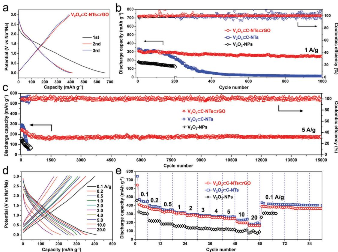
**Figure 6.** Sodium-ion-storage performance. a) Charge–discharge curves of the  $V_2O_3$ C-NTsCrGO anode from 0.01 to 3.0 V at 0.1 A g<sup>-1</sup> in different cycles. Cycling performance and corresponding coulombic efficiency of  $V_2O_3$ C-NTsCrGO,  $V_2O_3$ C-NTs, and  $V_2O_3$ -NPs at b) 1 A g<sup>-1</sup> and c) at high rate of 5.0 A g<sup>-1</sup> (initially activated at 0.1 A g<sup>-1</sup> for 3 cycles). d, e) Rate performance of the three samples at various current densities.
