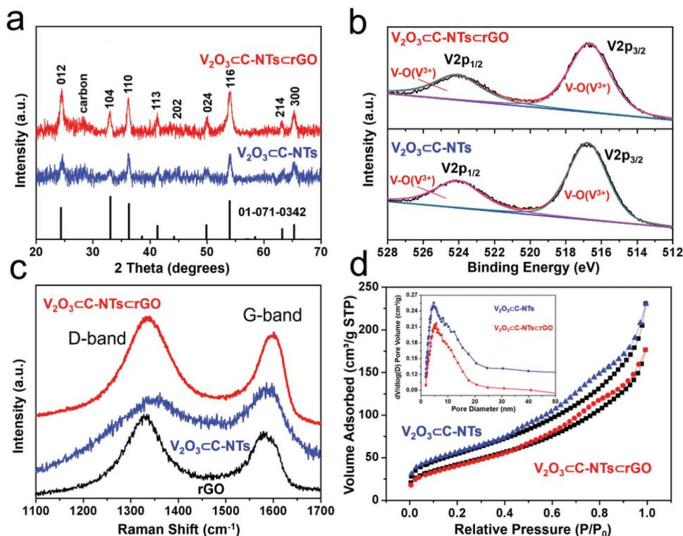
**Figure 3.** Phase, composition and pore structure characterization of  $V_2O_3C-NTsCrGO$  and  $V_2O_3C-NTs$ . The inset is the corresponding pore size distribution.
