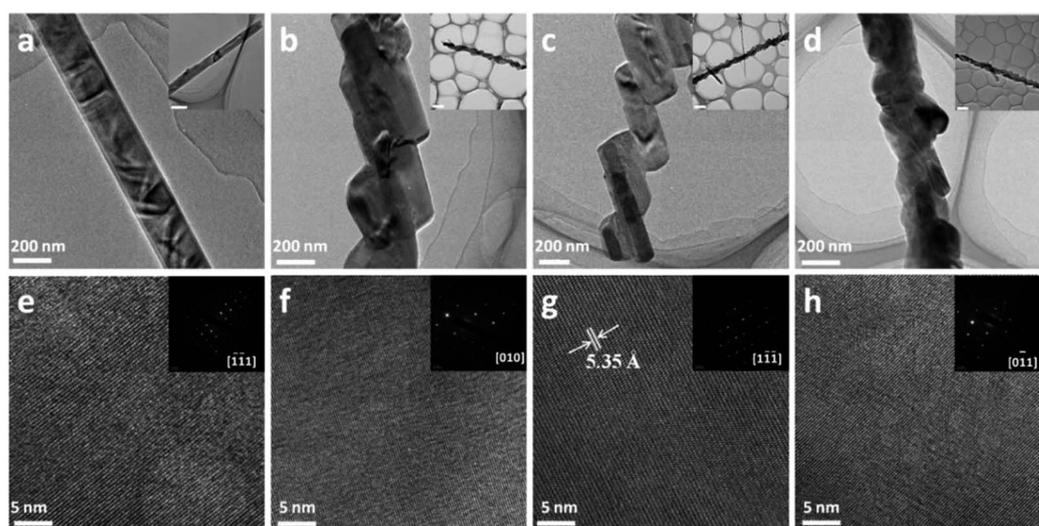
Fig. 3 Morphologies of products synthesized with different amounts of CTAB. TEM images of simple NVO (a), NVO-C1 (b), NVO-C2 (c) and NVO-C3 (d), and the insets in (a–d) show the morphologies in different scales (scale bar for a inset: 200 nm; for b–d insets: 1  $\mu\text{m}$ ). HRTEM images of simple NVO (e), NVO-C1 (f), NVO-C2 (g) and NVO-C3 (h), and the corresponding SAED patterns are shown in the insets of (e–h) with zone axis indicated.
