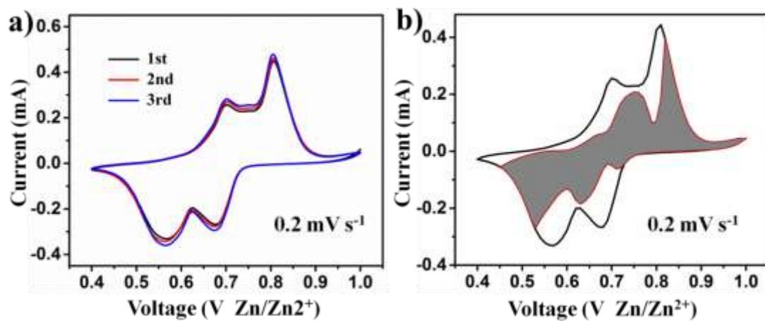
Figure S5. a) The CV curves of VS<sub>2</sub> at a scan rate of 0.1 mV/s, b) The contribution ratio of the capacitive capacities and diffusion-limited capacities at 0.1 mV/s.
