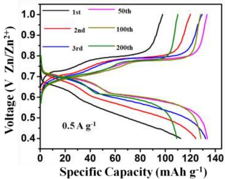
Figure S4. The charge and discharge curves of VS<sub>2</sub> of different cycles at a current density of 0.5 A g<sup>-1</sup>.
