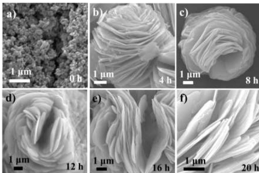
Figure S2. The growth process of VS<sub>2</sub> nanosheets at different reaction times (from 0 h to 20 h).
