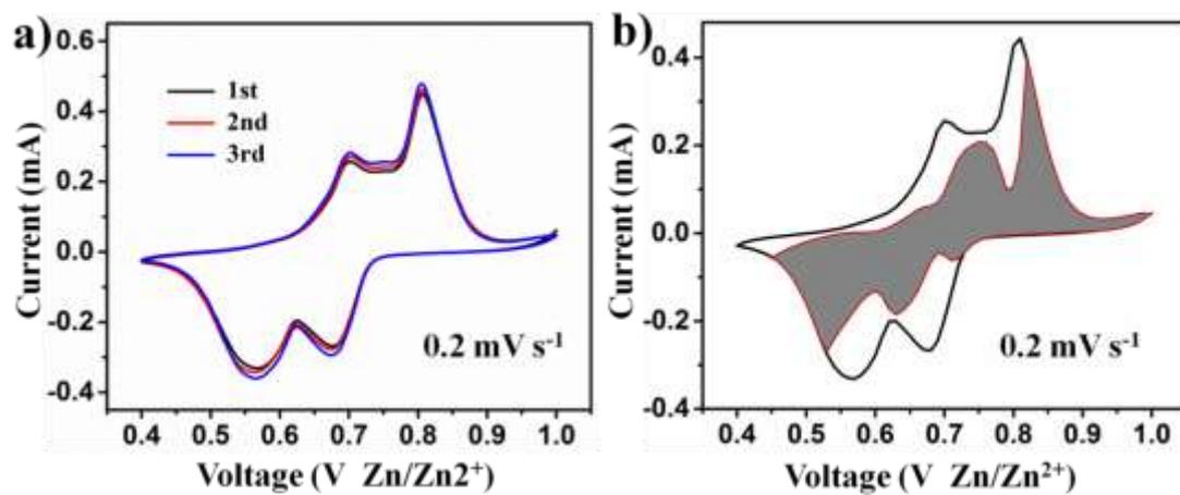
Figure S5. a) The CV curves of  $\text{VS}_2$  at a scan rate of  $0.1 \text{ mV/s}$ , b) The contribution ratio of the capacitive capacities and diffusion-limited capacities at  $0.1 \text{ mV/s}$ .
