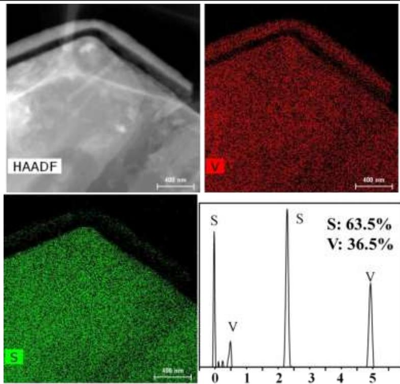
Figure S1. TEM-EDS of VS<sub>2</sub> nanosheets
