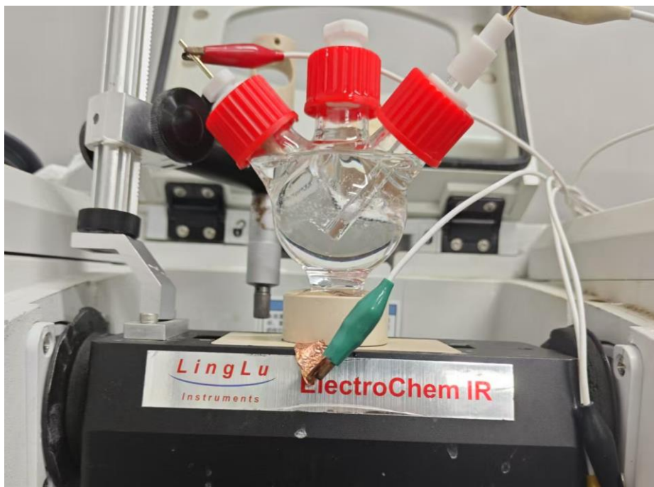
Supplementary Fig. 50 | Optical photograph for in-situ ATR-SEIRAS measurements.
