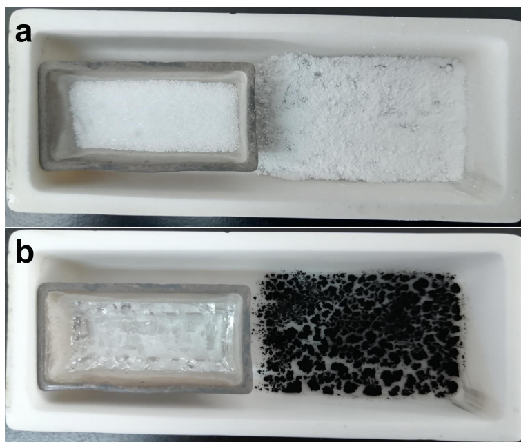
Supplementary Fig. 2. The photographs during the synthetic procedure of the Zn-SA/CNCl-1000 catalyst. a , 3 g NaCl in a smaller ceramic boat and 150 mg ZIF-8 powder were put together in a larger ceramic boat with a lid. b , After pyrolysis at 1000°C (heating rate: 5°C/min) for 3 h under flowing argon gas (99.999%), the black Zn-SA/CNCl-1000 powder was obtained.
