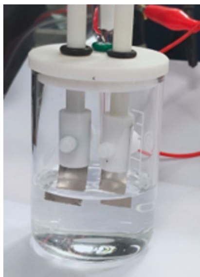
Figure S9. LSV test images of current collectors in three-electrode cells.
