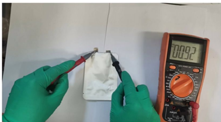
Figure S34. Open the current potential of OPMO//CuFe-TBA full battery after the first charge.
