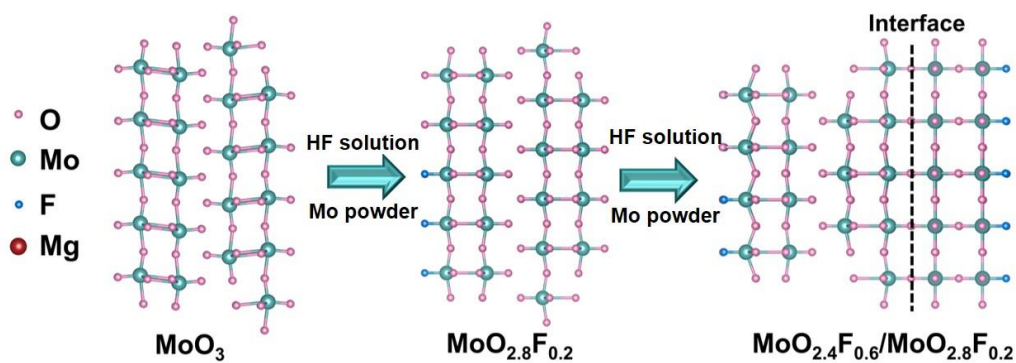
Figure S6. Schematic illustration of synthesis process of o-c \text{MoO}_{2.8}\text{F}_{0.2}/\text{MoO}_{2.4}\text{F}_{0.6} heterostructures.
