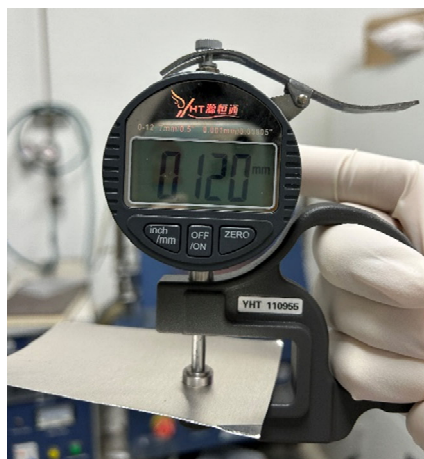
Figure S30 The thickness of the Mg sheet used in pouch cells
