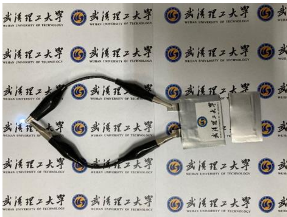
Figure S28. LiFePO 4 /CPDOL-SPE/Li pouch battery after cutting.
