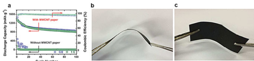
Fig. 4.33 a Cycle performance of high-rate Li-S batteries armed with and without the MWCNT insertion between separator and cathode, respectively. b, c Digital photos of the CNF-TiO 2 (CNF-T) interlayer under mechanical bending conditions. Panels adapted with permission from: a Ref. [61], RSC; b, c, d Ref. [62], ACS
