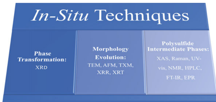
Fig. 9.1 Different in situ characterization techniques for understanding the reactions in Li-S battery
