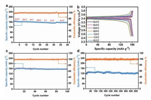
Figure 4. Electrochemical performances of Li/CSIL/LFP solid-state batteries. a) Cycling stability with Coulombic efficiency under different current rates 0.2, 0.4, 0.6, 0.8, 1.0, 1.5, and 0.2 C. b) Typical charge/discharge profiles at different current rates. c,d) Cycling stability with Coulombic efficiency under 0.2 and 3 C. All tests were conducted at room temperature.
