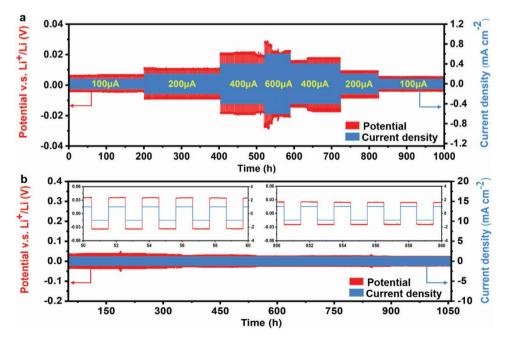
Figure 3. a) Voltage profile of the Li/CSIL/Li symmetric batteries at different current densities (100 200, 400, and 600  $\mu$ A cm<sup>-2</sup>). b) Voltage profile of the Li/CSIL/Li symmetric battery at a current density of 1000  $\mu$ A cm<sup>-2</sup> Insets: Detailed voltage profiles of the 50–60 and 850–860 h, respectively. All tests were performed at room temperature.
