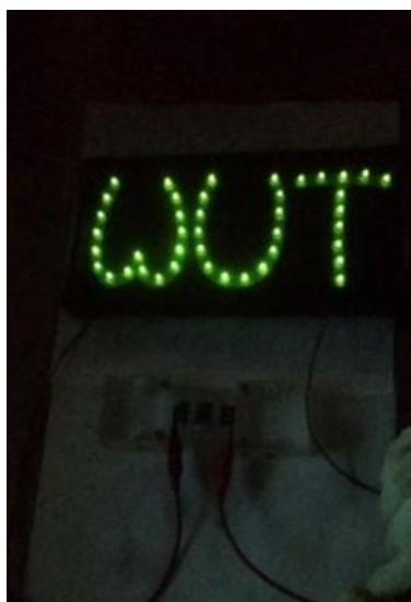
Figure S15. Photograph of three Co-Zn microbatteries connected in series for lighting an LED scroller of “WUT” log.
