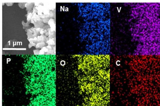
**Figure S2.** Energy dispersive spectrometry elemental mapping of NVP/C.
