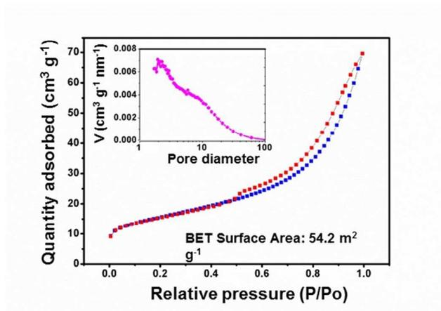
**Figure S4.** Nitrogen adsorption-desorption isotherms (inset is the corresponding pore size distribution) of NVP/C.
