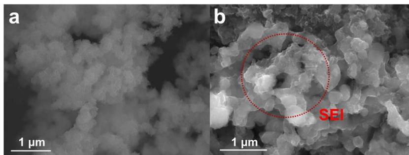
**Figure S6.** The morphological of (a) the NVP/C materials and (b) the anode material with pre-intercalation.
