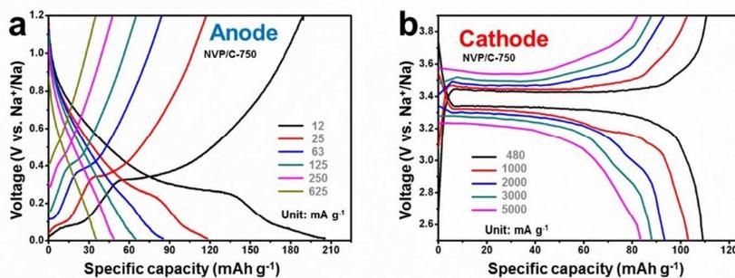
Figure S9. Typical voltage profiles of NVP/C as (a) cathode and (b) anode in different current densities.
