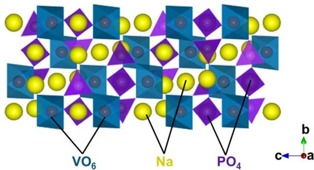
**Figure S1.** Crystal structure of Na<sub>3</sub>V<sub>2</sub>(PO<sub>4</sub>)<sub>3</sub> (NVP).
