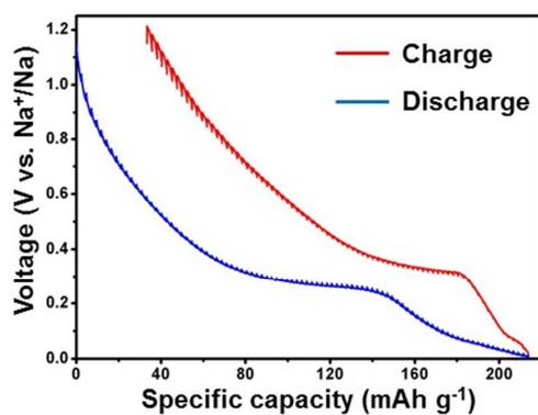
Figure S7. The GITT curves of  $\text{Na}_4\text{V}_2(\text{PO}_4)_3$  in the third cycle.
