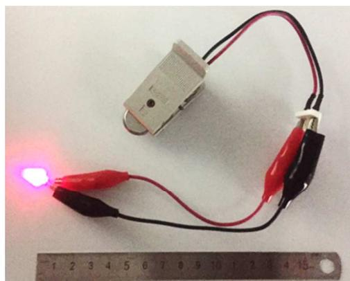
**Figure S11.** The lighted LED bulb driven by the full cell.
