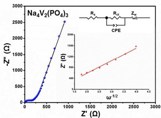
Figure S8. EIS results of  $\text{Na}_4\text{V}_2(\text{PO}_4)_3$  electrode, inset is the calculation of Warburg factor.
