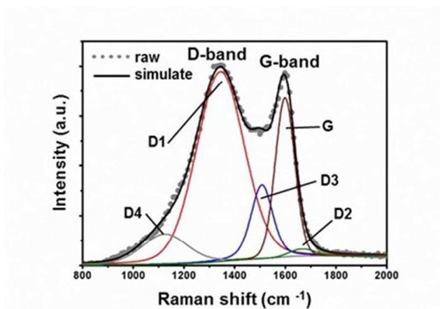
**Figure S3.** Raman spectrum of NVP/C.
