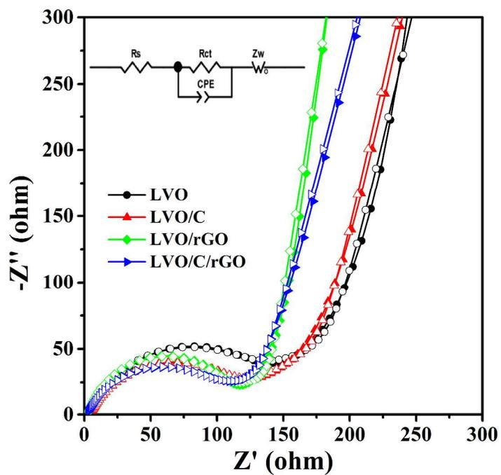
**Figure S10.** EIS spectra of LVO, LVO/C, LVO/rGO, and LVO/C/rGO.
