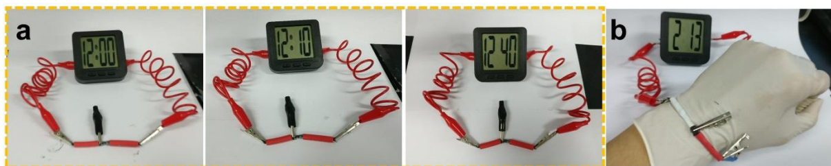
Figure S25. a) A digital watch was powered by two-in-series battery. b) A digital watch was powered by a bracelet battery.
