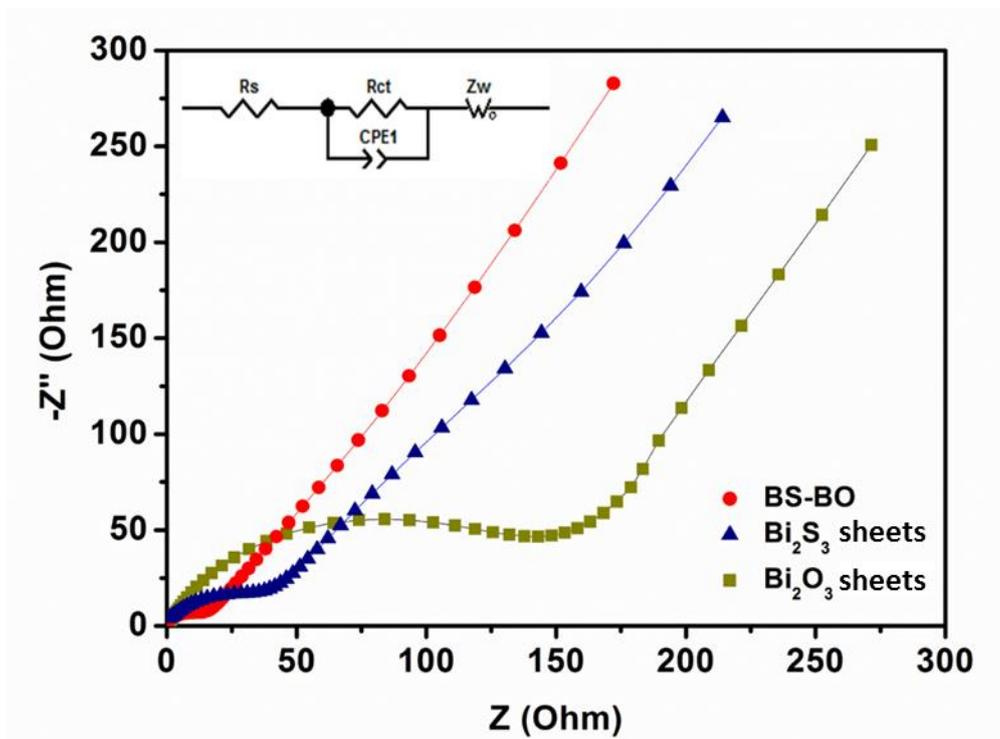
**Figure S10** Nyquist plots of electrodes containing BS-BO, Bi<sub>2</sub>S<sub>3</sub> sheets and Bi<sub>2</sub>O<sub>3</sub> sheets. The equivalent circuit is inset.
