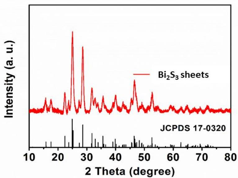
**Figure S1** XRD pattern of Bi<sub>2</sub>S<sub>3</sub> sheets.
