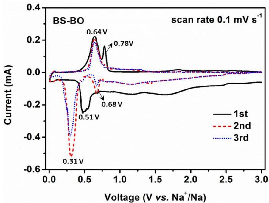
**Figure S5** Cyclic voltammograms for the first three cycles of BS-BO electrode in SIBs at a scan rate of 0.1 mV s<sup>-1</sup>.
