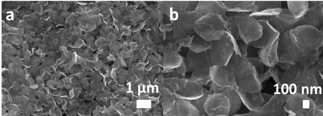
**Figure S4** SEM images of Bi<sub>2</sub>S<sub>3</sub> sheets at low (a) and high (b) magnifications.
