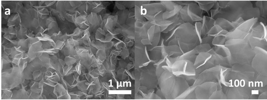
**Figure S3** SEM images of Bi<sub>2</sub>O<sub>3</sub> sheets at low (a) and high (b) magnifications.
