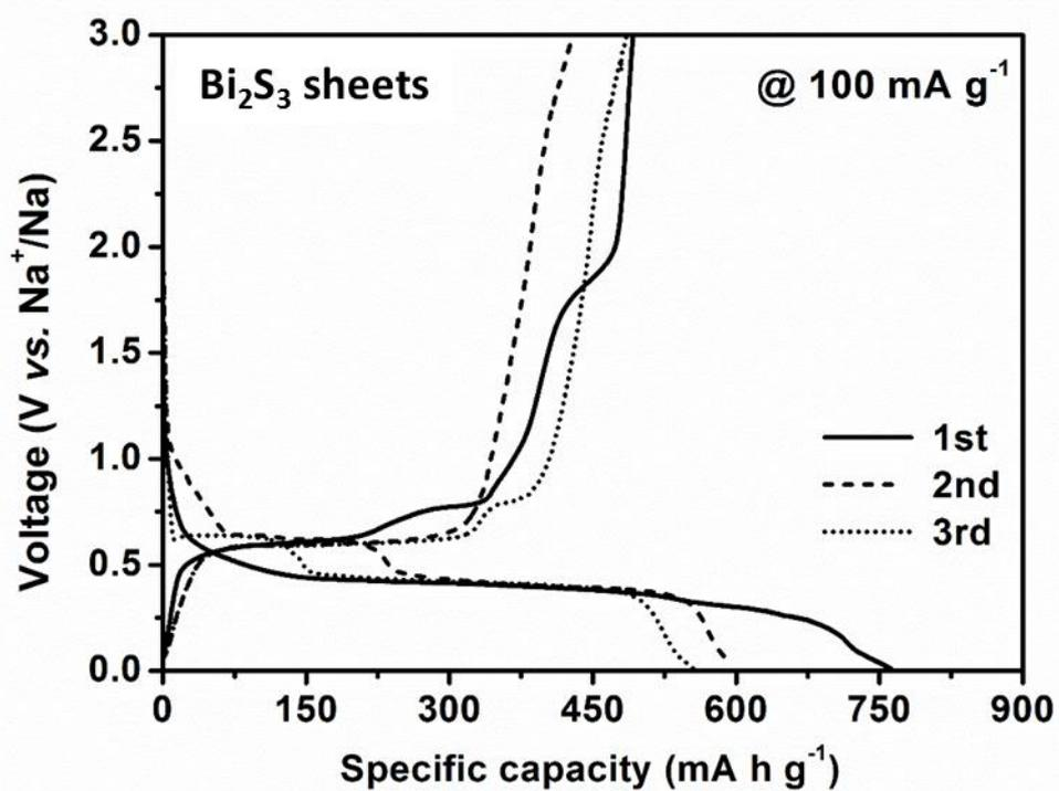
**Figure S8** The typical charge/discharge profiles of Bi<sub>2</sub>S<sub>3</sub> sheets at the current density of 100 mA g<sup>-1</sup> for the initial three cycles.
