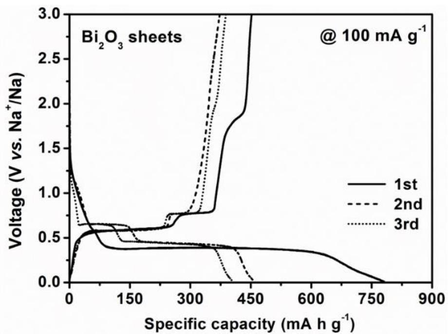
**Figure S9** The typical charge/discharge profiles of Bi<sub>2</sub>O<sub>3</sub> sheets at the current density of 100 mA g<sup>-1</sup> for the initial three cycles.
