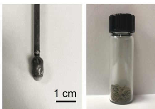
Figure S3. Photographs of the silicon product from the electrolysis reaction using \text{CaSiO}_3 + \text{CaCl}_2 salts under 850^\circ\text{C} after a 3 h electrolysis under 1.6 V (reaction 1 in Table S1).
