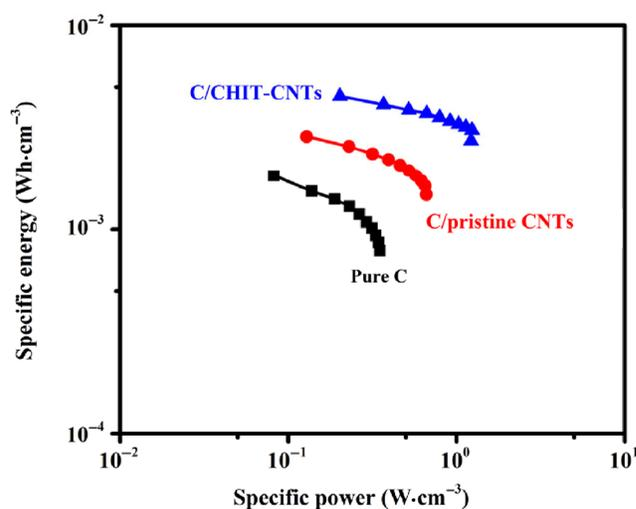
**Figure 5** Ragone plots of the volumetric energy and power density of the fabricated micro-supercapacitors with different microelectrodes.
