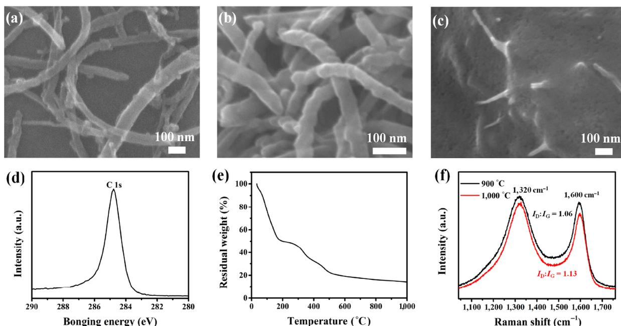
**Figure 2** SEM images of (a) pristine CNTs, (b) CHIT-CNTs, and (c) C/CHIT-CNT microelectrodes after pyrolysis at  $900\text{ }^{\circ}\text{C}$ . (d) High-resolution XPS spectrum in the C 1s region of the pyrolyzed carbon microelectrodes after pyrolysis at  $900\text{ }^{\circ}\text{C}$ . (e) TGA curve of the PR1-9000A photoresist. (f) Raman spectra of the samples after pyrolysis at 900 and  $1,000\text{ }^{\circ}\text{C}$ .
