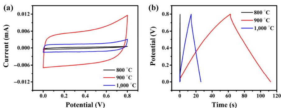
**Figure 3** (a) CV curves of the C/CHIT-CNT microelectrode-based micro-supercapacitor at a scan rate of  $10 \text{ mV}\cdot\text{s}^{-1}$ . (b) Galvanostatic charge–discharge profile of C/CHIT-CNT microelectrode-based micro-supercapacitor at a current density of  $0.1 \text{ mA}\cdot\text{cm}^{-2}$ .
