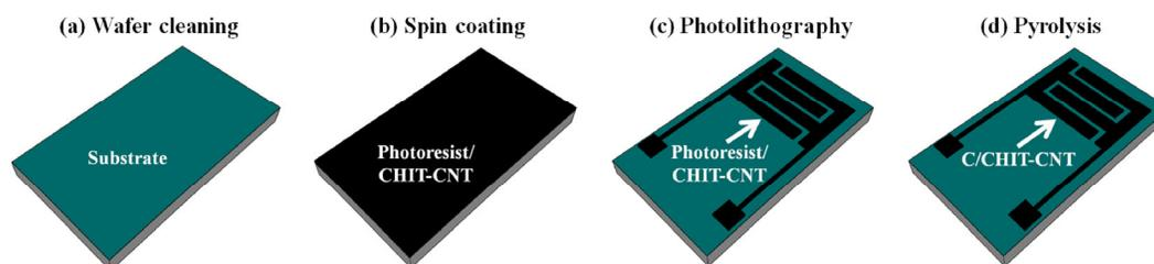
**Figure 1** Microfabrication process of the C/CHIT-CNT micro-supercapacitor. (a) RCA cleaning of the Si/SiO<sub>2</sub> substrate. (b) Spin coating of photoresist/CHIT-CNT composite on the substrate. (c) Photolithography, development, and rinse. (d) Pyrolysis.
