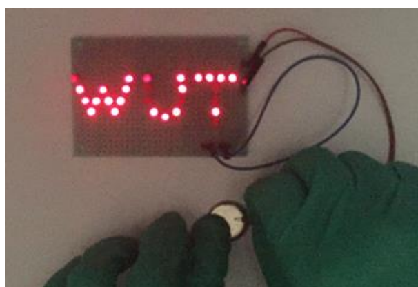
Figure S11. Digital image of a light-emitting diode lit by SnO 2 QDs@GO/LiFePO 4 lithium ion battery.
