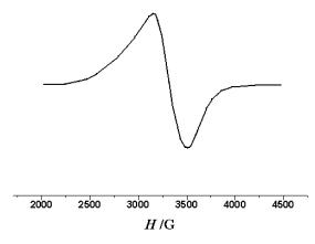
Fig. 4. ESR spectrum of vanadium oxide nanotubes.
